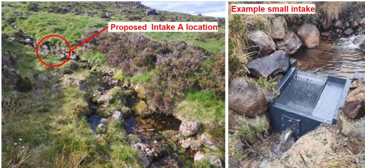
Figure 4 - Proposed Intake A location: NG 99775 51643 (Left), example small powder coated intake box (right)
