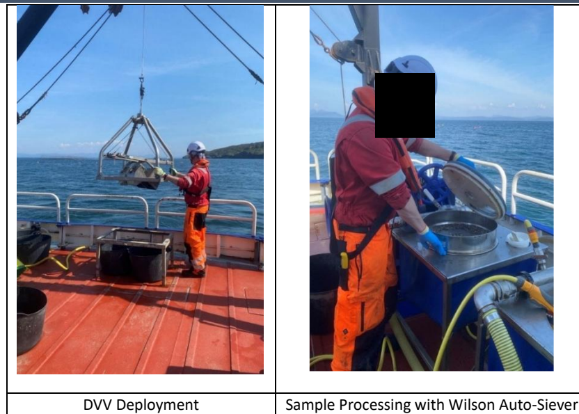
Figure 2-3 Dual Van Veen Grab Deployment and Fauna Sample Processing
