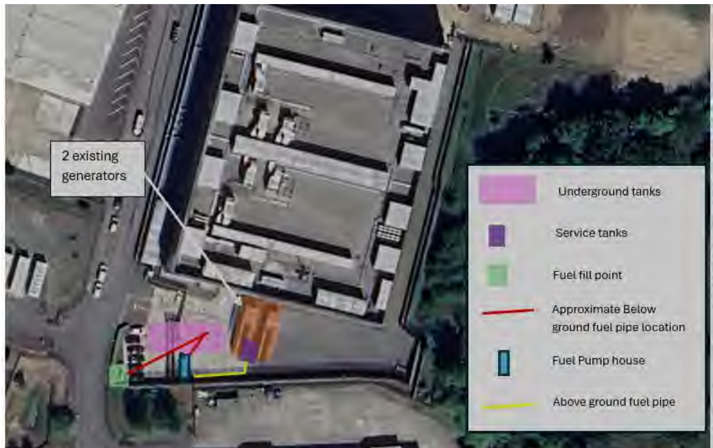
Figure 2: Approximate Fuel Transport Arrangements on Site
