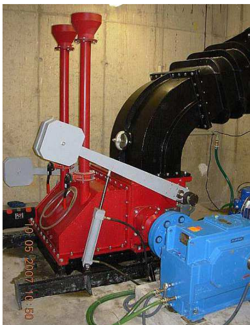
Figure 5 : Crossflow turbine unit (vertical inlet), plus schematic illustration
