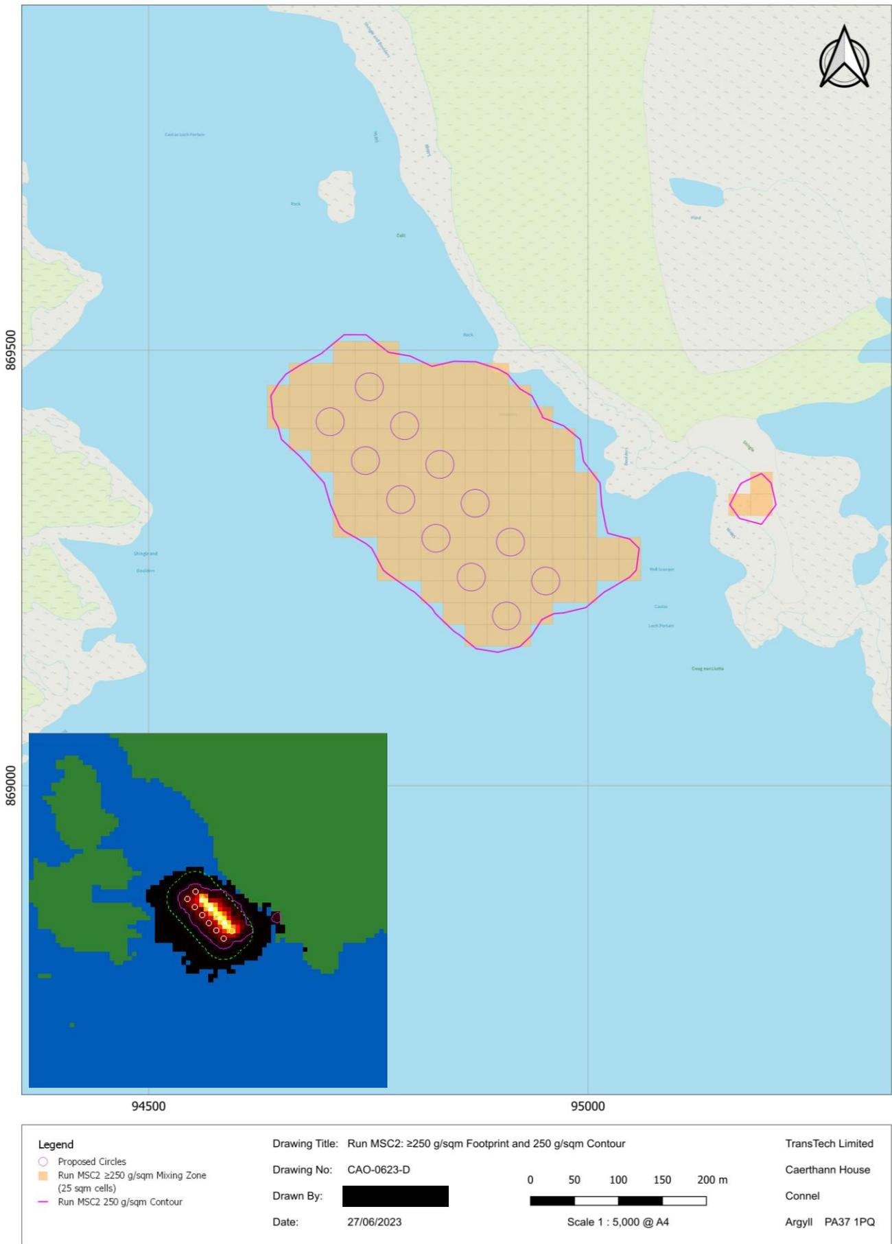
Figure 8. Run MSC2 (average for days 275-365): 250 g/m<sup>2</sup> modelled footprint and this run's 88,750 m<sup>2</sup> mixing zone area along with the UI's display of this.
