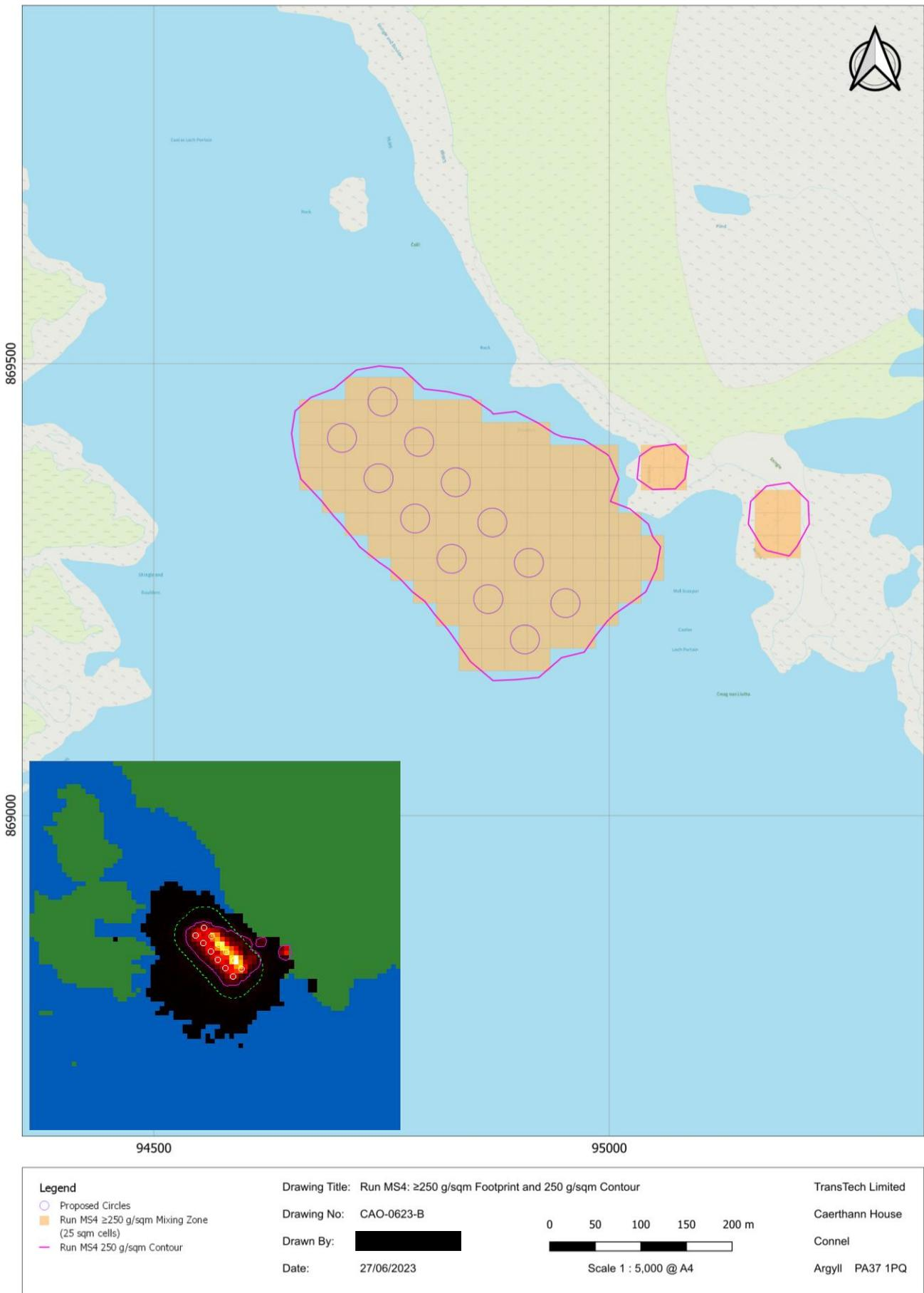
Figure 5. Run MS4 (average for days 275-365): 86,875 m<sup>2</sup> mixing zone area and 250 g/m<sup>2</sup> contour. UI plot also shown.
