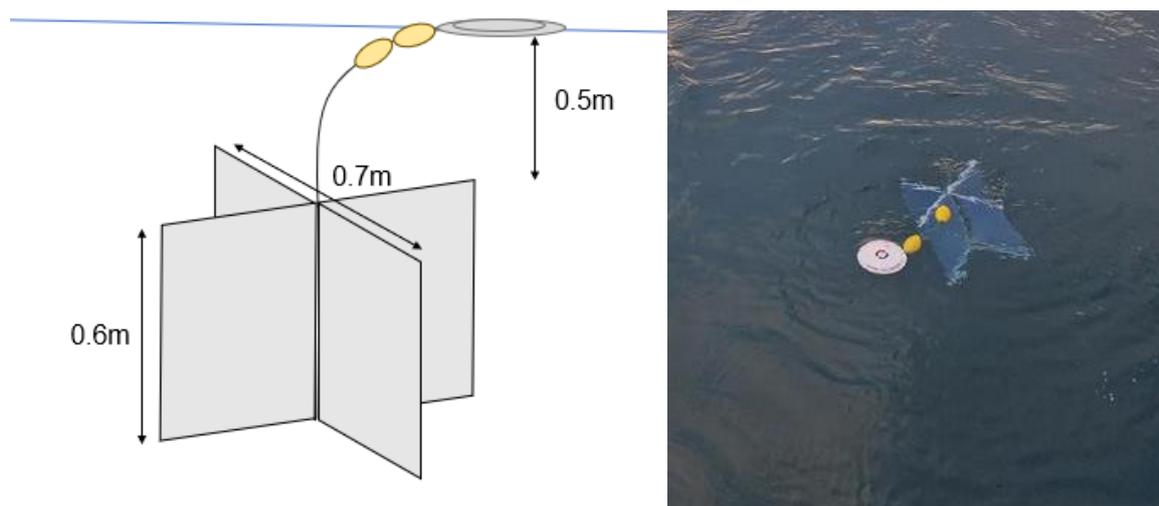
Figure 5. (left) Diagram of drogue with measurements. (right) Photo of drogue sinking immediately after deployment.
