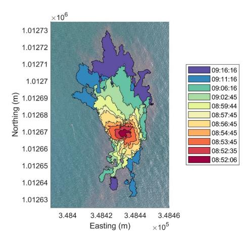
Figure 6. Extent of mapped dye plume boundary from a selection of timesteps from R4.
