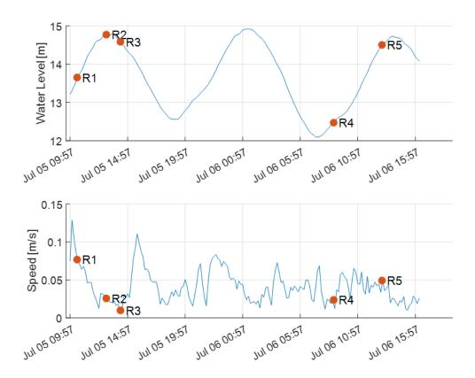
Figure 2. Tidal elevation and near-surface current velocity with the dye release times.
