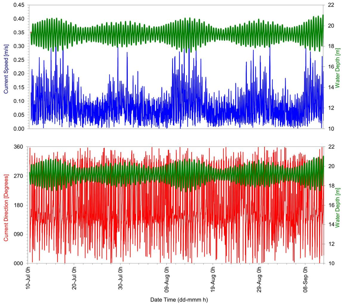
Figure 6.12 Sub-surface time series plots for current speed and direction against water level.
