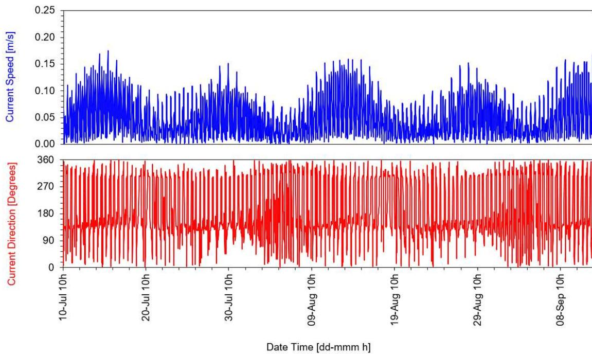
Figure 6.9 Near-bed time series plots for harmonic reproduction of speed and direction.
