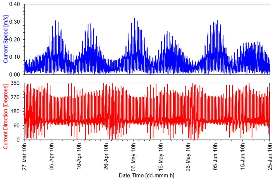
Figure 6.2 Near-bed time series plots for harmonic reproduction of speed and direction.
