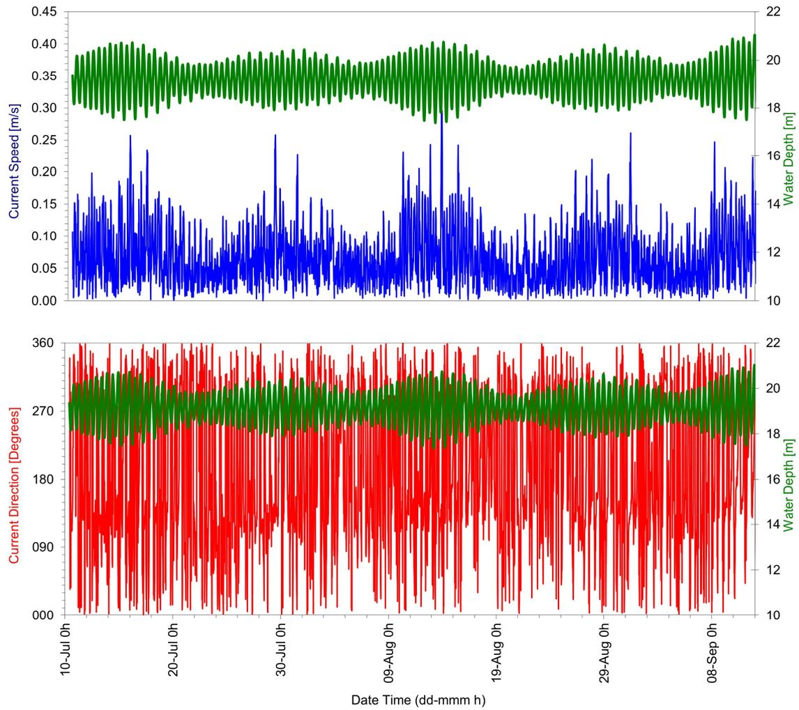
Figure 6.8 Near-bed time series plots for current speed and direction against water level.
