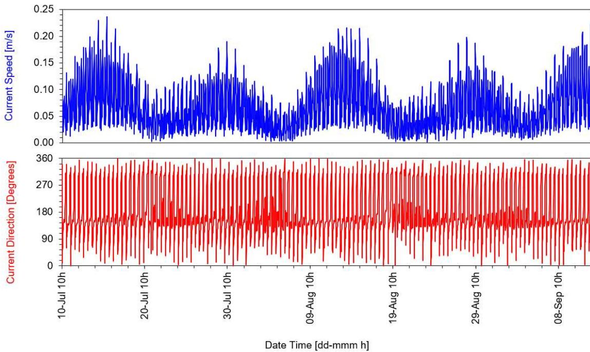
Figure 6.11 Pen-bottom time series plots for harmonic reproduction of speed and direction.
