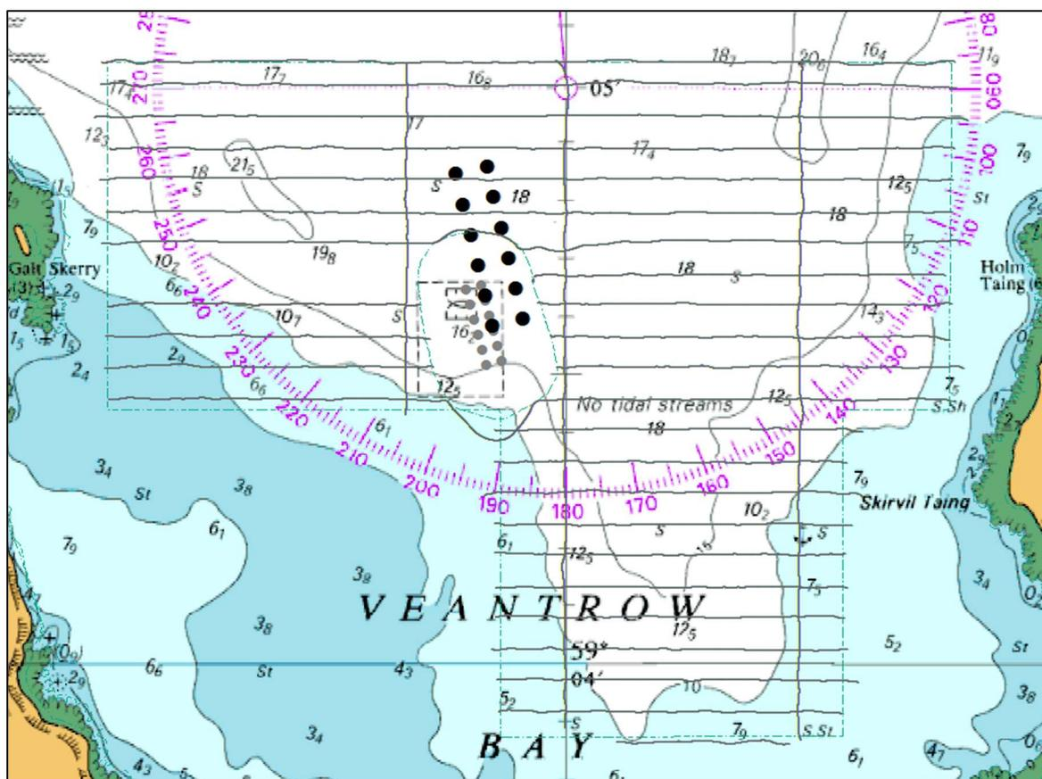
Figure 5.1 Plot of the vessel track from the 2018 multibeam survey at Veantrow Bay including existing (grey) and proposed pens (black).
