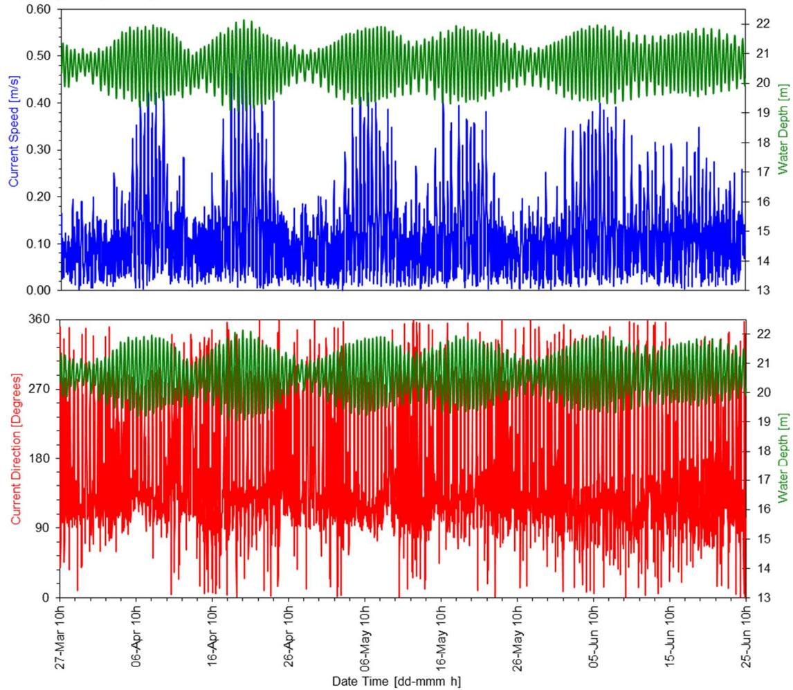
Figure 6.5 Sub-surface (bin 14) time series plots for current speed and direction against water level.
