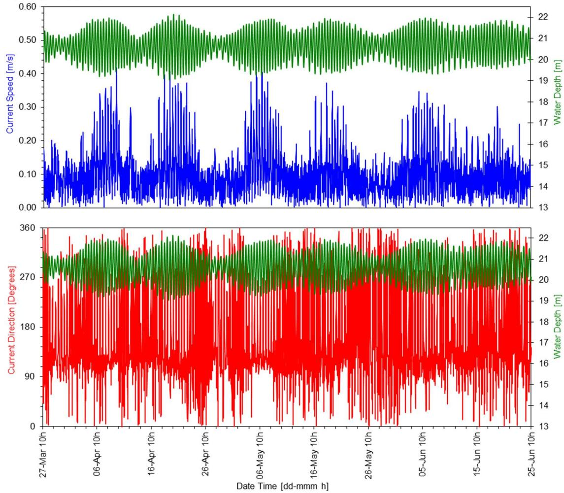
Figure 6.1 Near-bed time series plots for current speed and direction against water level.
