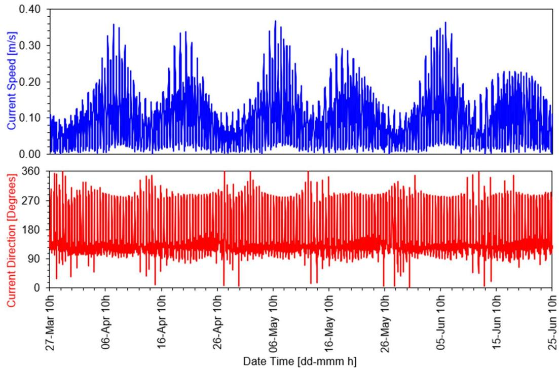
Figure 6.4 Pen-bottom time series plots for harmonic reproduction of speed and direction.
