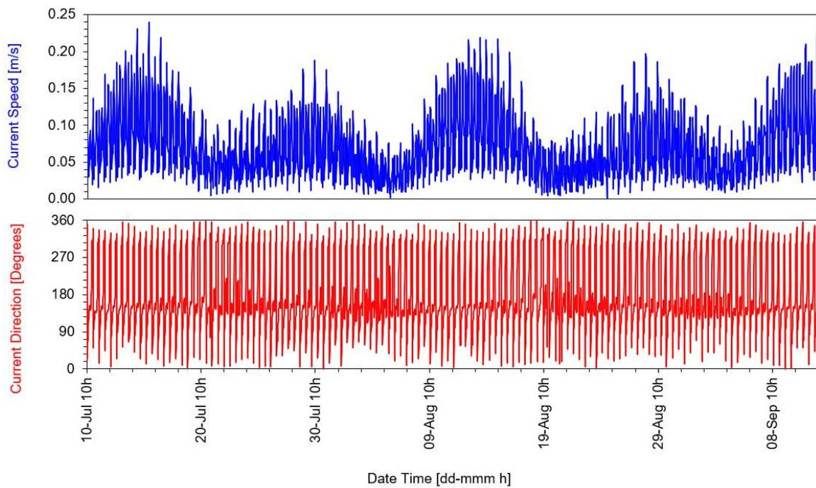
Figure 6.13 Sub-surface time series plots for harmonic reproduction of speed and direction.
