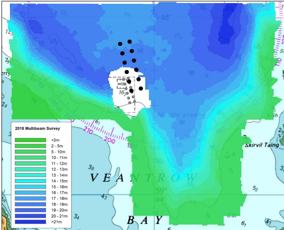
Figure 5.2 Plot of the interpolated bathymetry from the 2018 multibeam survey at Veantrow Bay including existing (grey) and proposed pens (black).
