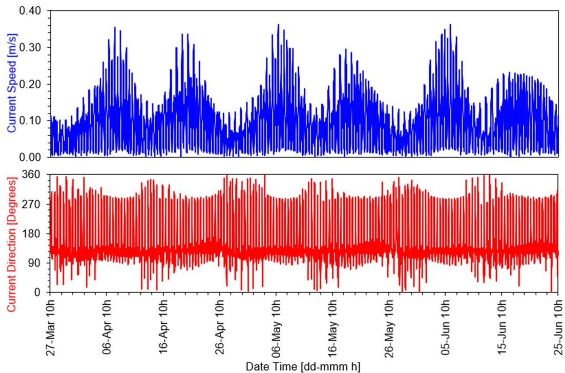
Figure 6.6 Sub-surface (bin 14) time series plots for harmonic reproduction of speed and direction.
