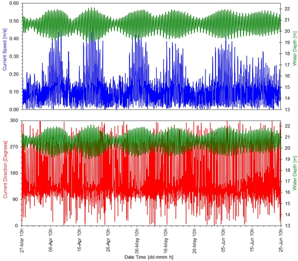
Figure 6.3 Pen-bottom time series plots for current speed and direction against water level.
