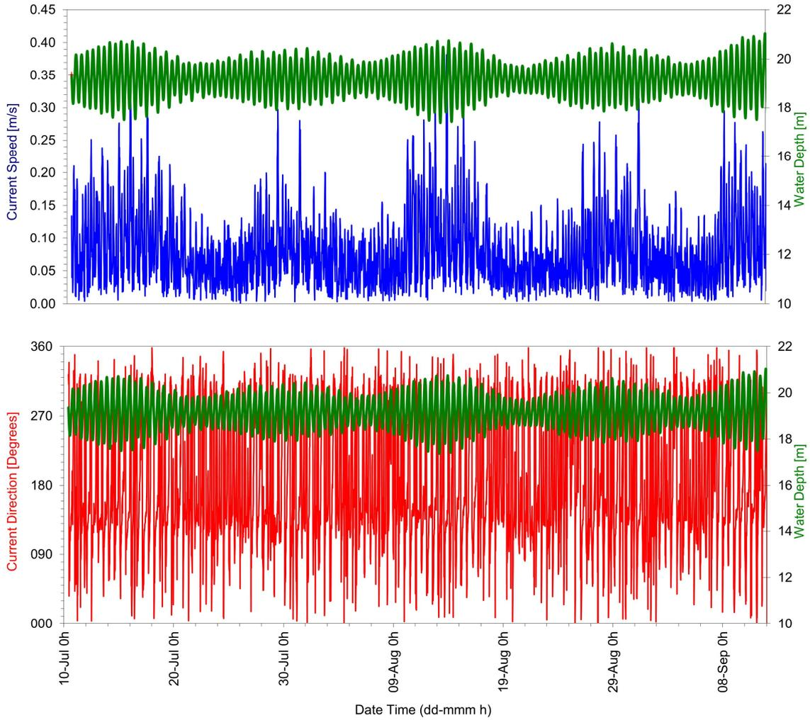
Figure 6.10 Pen-bottom time series plots for current speed and direction against water level.
