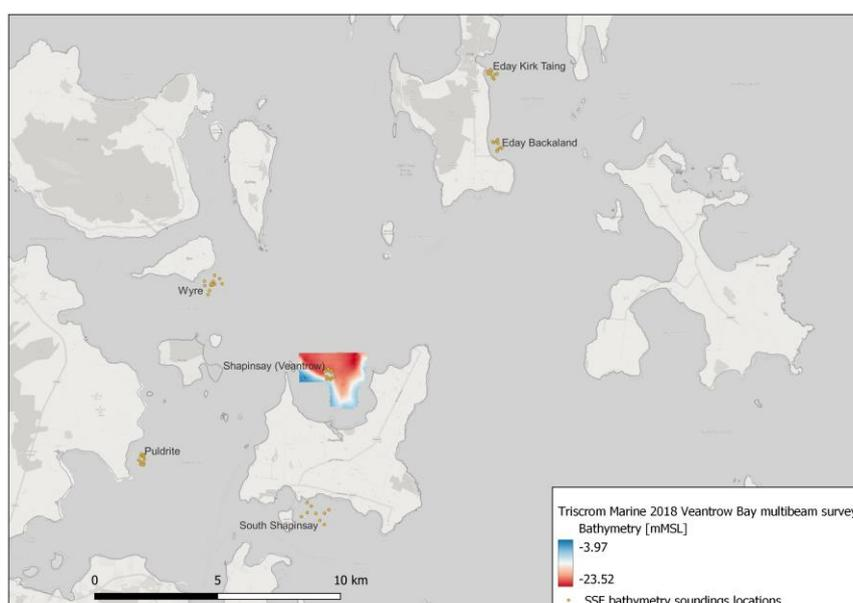
Figure 3.1 Map showing locations of bathymetry soundings (orange markers) at MPFF sites and multibeam survey at Veantrow Bay provided by SSF.
