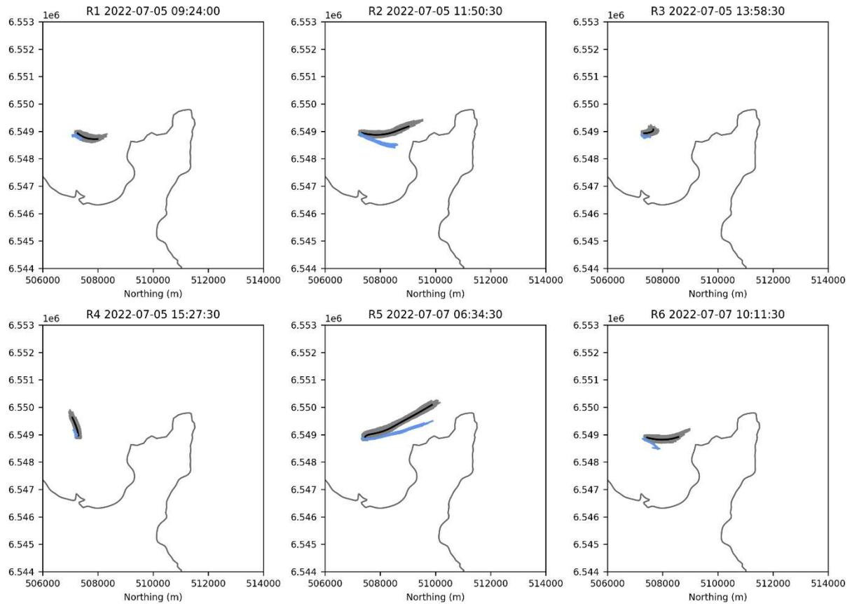
Figure 5.3: Wind (weighting 0.01), simulation release 45 minutes earlier. Drogue tracks (blue) overlaid on a sample of 100 model particle tracks (grey), and the mean of all model tracks for that release (black).
