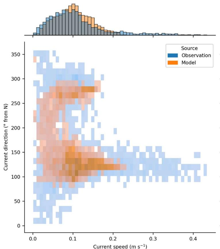
Figure 4.7: Histogram of speed versus direction for current meter observation (depth averaged, blue) and model prediction for the selected period (orange).
