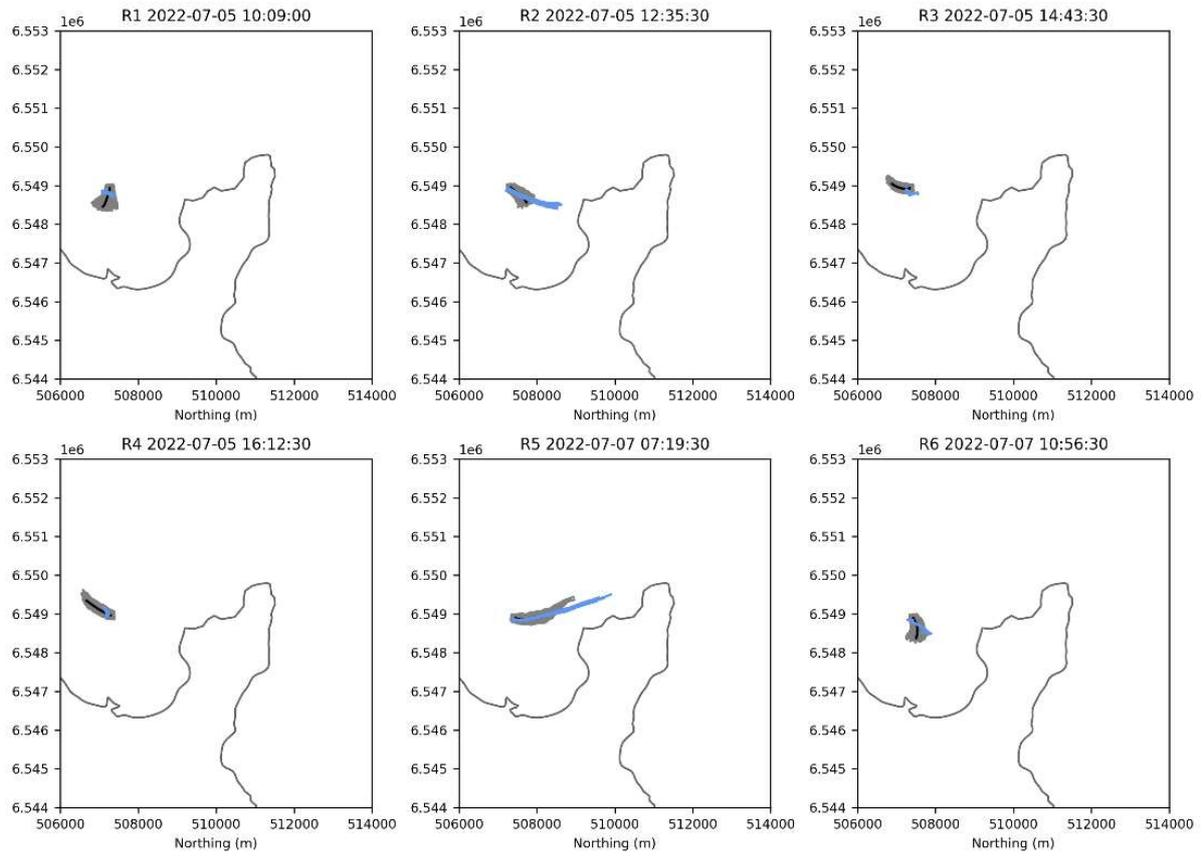
Figure 5.1: No wind, no time offset. Drogue tracks (blue) overlaid on a sample of 100 model particle tracks (grey), and the mean of all model tracks for that release (black).
