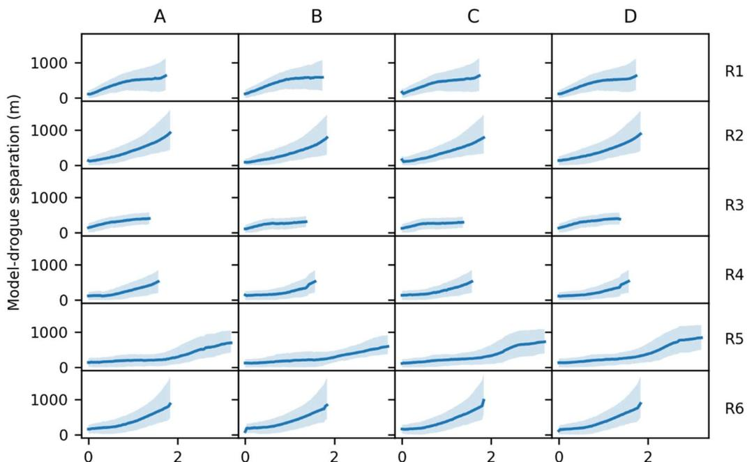
Figure 5.4: Wind (weighting 0.01), simulation release 45 minutes later. Distance between model particles and each drogue (columns A-D) within each release (rows R1-6). Dark blue line indicates the median particle distance to the specific drogue, light blue shading indicates minimum and maximum distance.
