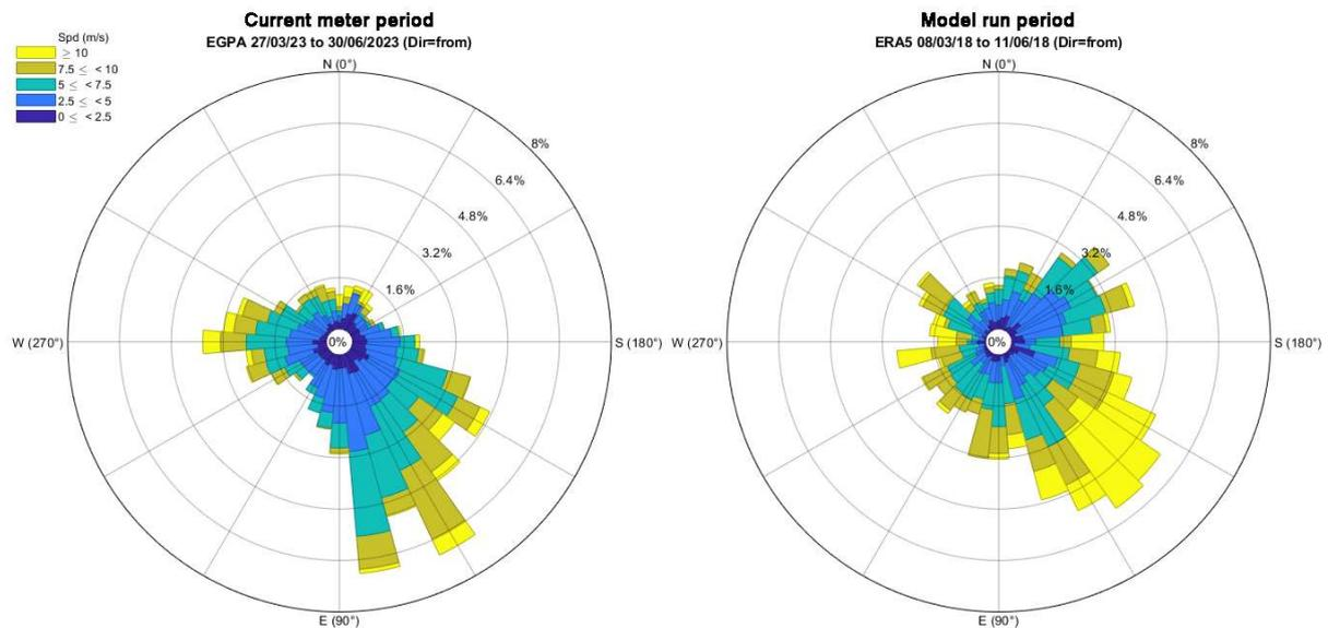
Figure 4.2: Wind roses showing speed and direction of wind observations at Kirkwall Airport (EGPA) during the current meter period (left) and the ERA5 data extracted for the selected model run period (right).
