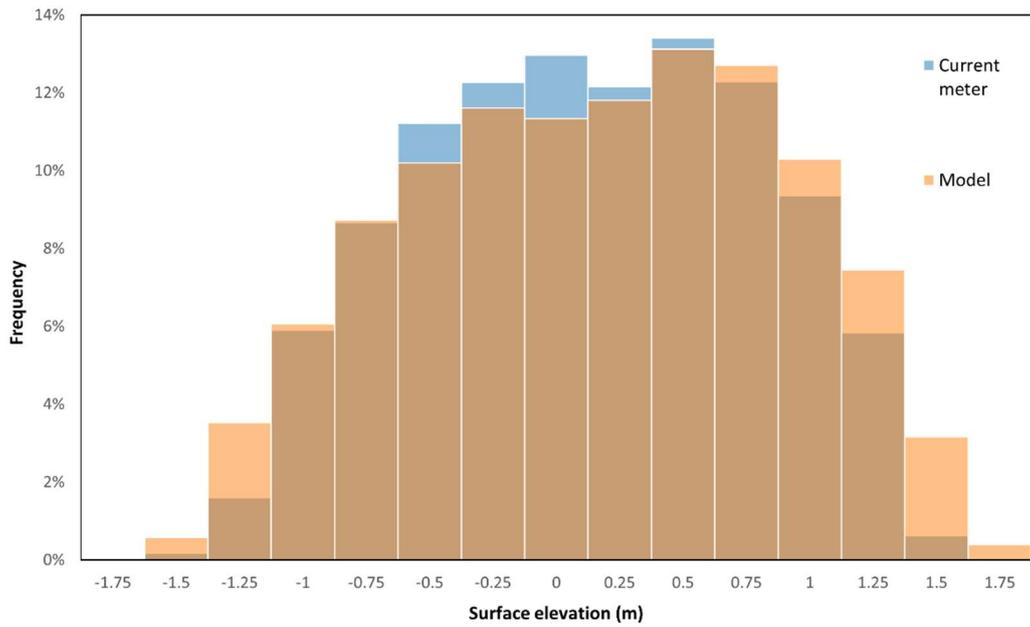
Figure 4.4: Water level comparison between current meter observation (blue) and HD model extract for the location (orange).
