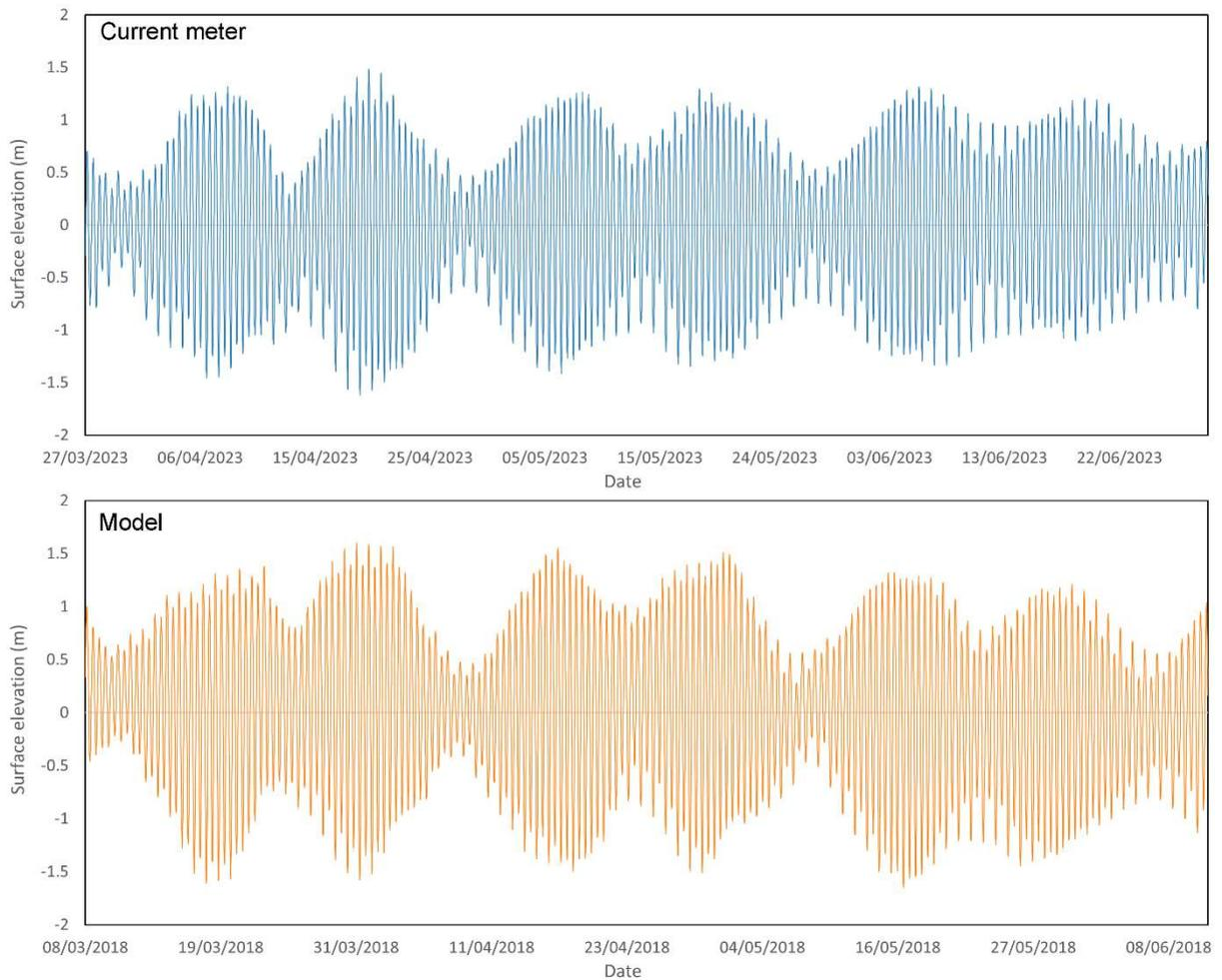
Figure 4.5: Surface elevation timeseries recorded by the current meter (blue), and for the selected model period (orange).
