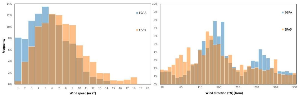
Figure 4.3: Histogram plots of wind speed (left) and direction (right) over the current meter observation period (blue, Kirkwall Airport (EGPA)) and selected model run period (orange, ERA5).
