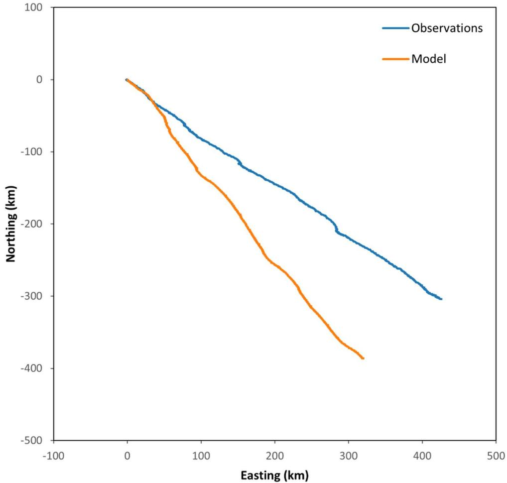
Figure 4.8: Progressive flow plot showing vectors generated from the current meter record (blue), and those from the model output (orange, lines matching direction from point (0,0) would indicate a good match).
