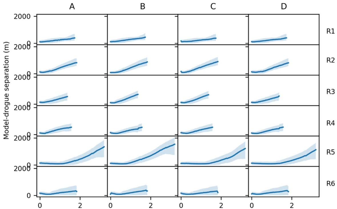
Figure 5.2: No wind, no time offset. Distance between model particles and each drogue (columns A-D) within each release (rows R1-6). Dark blue line indicates the median particle distance to the specific drogue, light blue shading indicates minimum and maximum distance.
