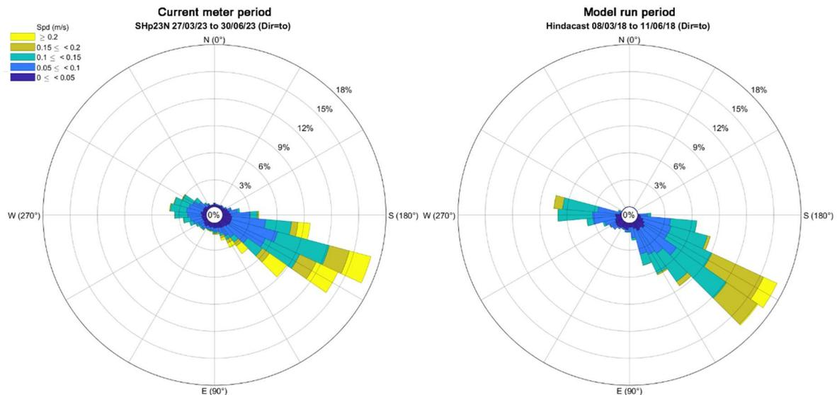
Figure 4.6: Current rose for current flows showing current meter observation (depth averaged, left) and model prediction for the selected period (right).
