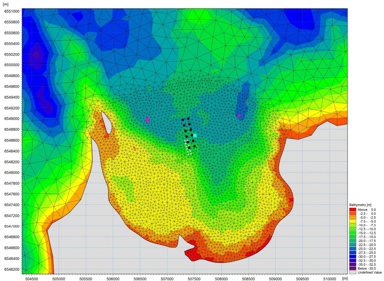
**Figure 3.2:** Close-up view of the computational mesh of Veantrow Bay. Existing validation current meter data sets used during the North Orkney hydrodynamic model build are indicated (magenta points), as well as the 2023 current meter deployment (cyan point), and the existing and proposed pens (grey and black points respectively).
