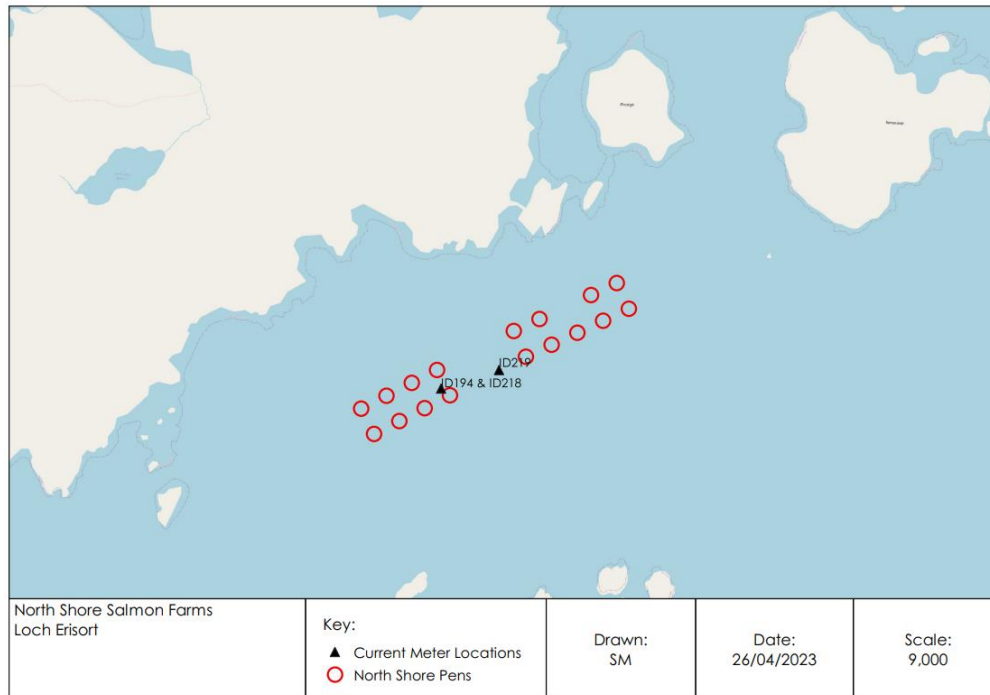
Figure 4. The current pen layouts at both North Shore East and North Shore West. Current meter positions are shown by the black triangles
