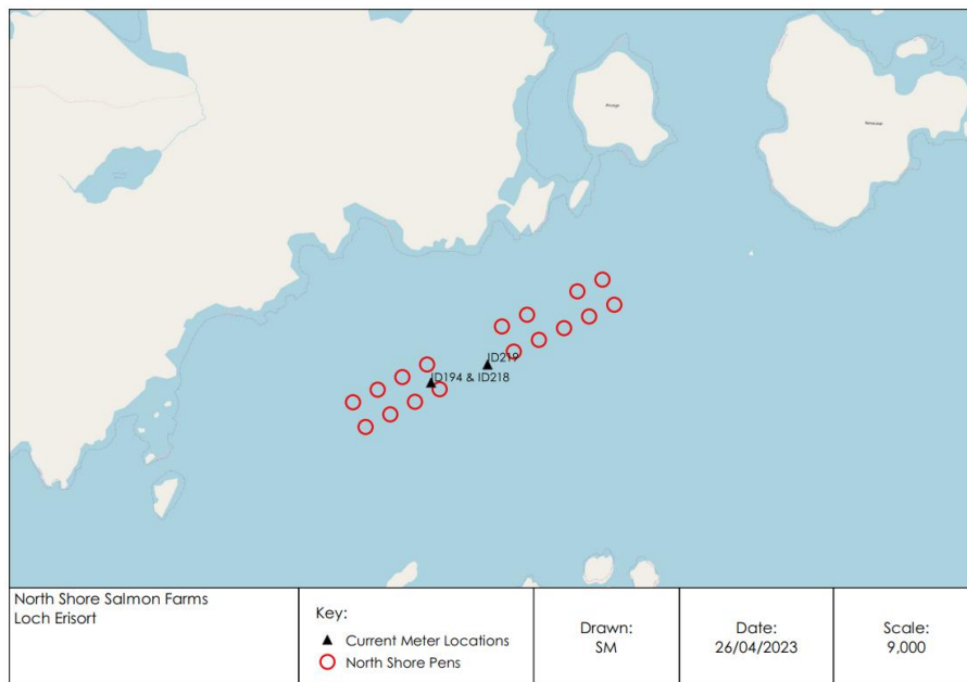
Figure 1. Location of the two salmon farms, North Shore West (left group) and the neighbouring site North Shore East (right group) and the location of the ADCP deployments (▲) relative to the pen positions (○).
