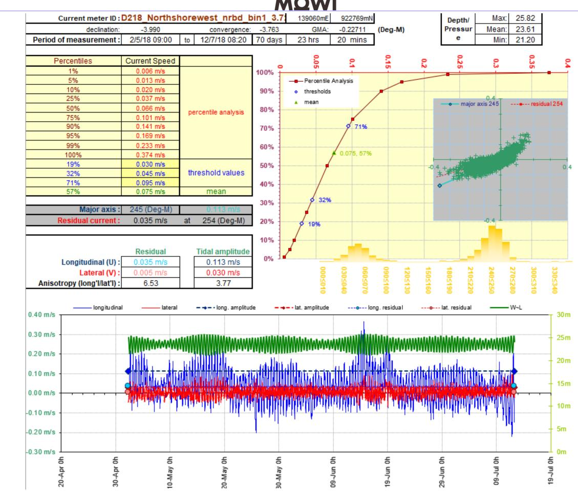
Figure 6. Current Data Summary Sheet for the near bottom current cell 1, 3.2 m from seabed, 2<sup>nd</sup> May to 12<sup>th</sup> July 2018 inclusive (ID218).
