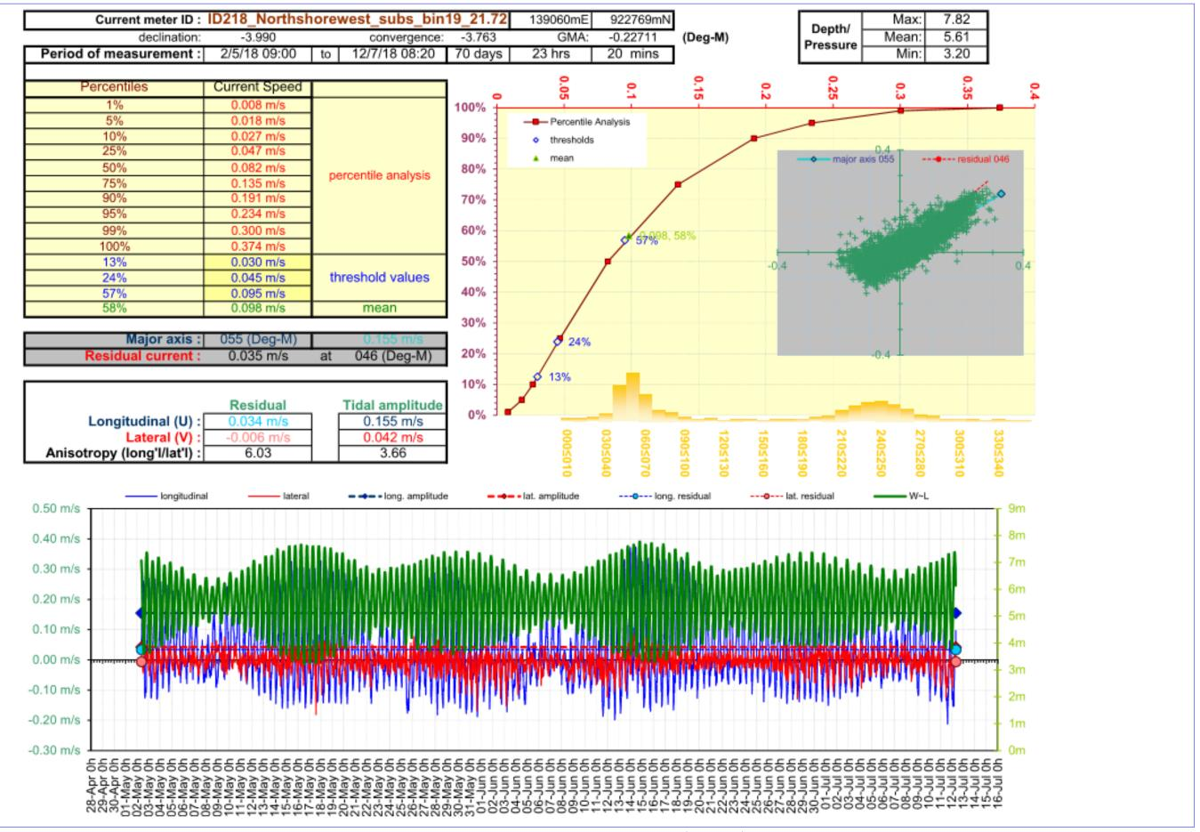
Figure 4. Current Data Summary Sheet for the surface current cell 19, 21.72 m from seabed, 2<sup>nd</sup> May to 12<sup>th</sup> July 2018 inclusive (ID218).
