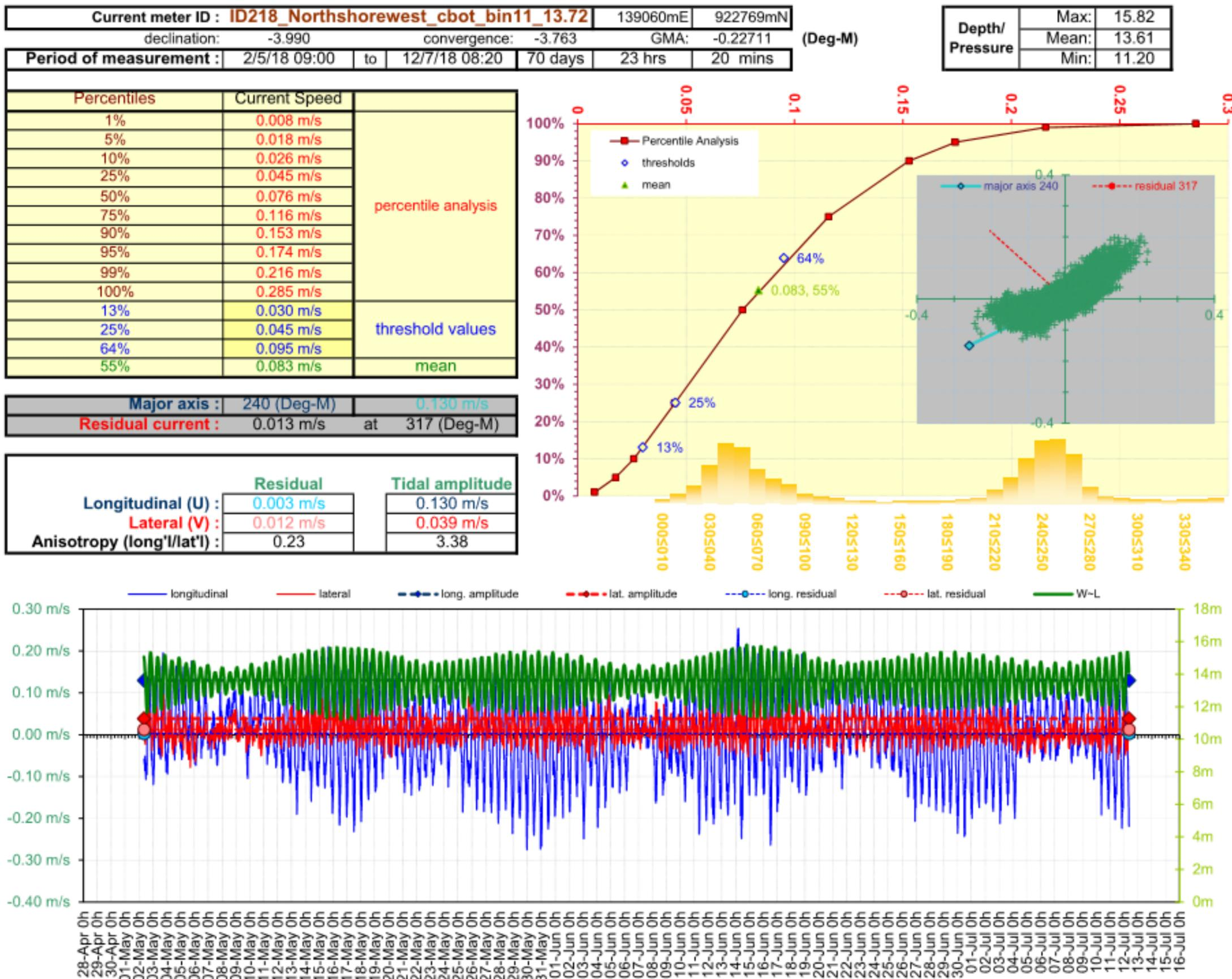
Figure 5. Current Data Summary Sheet for the cage bottom current cell 11, 13.72 m from seabed, 2<sup>nd</sup> May to 12<sup>th</sup> July 2018 inclusive (ID218).
