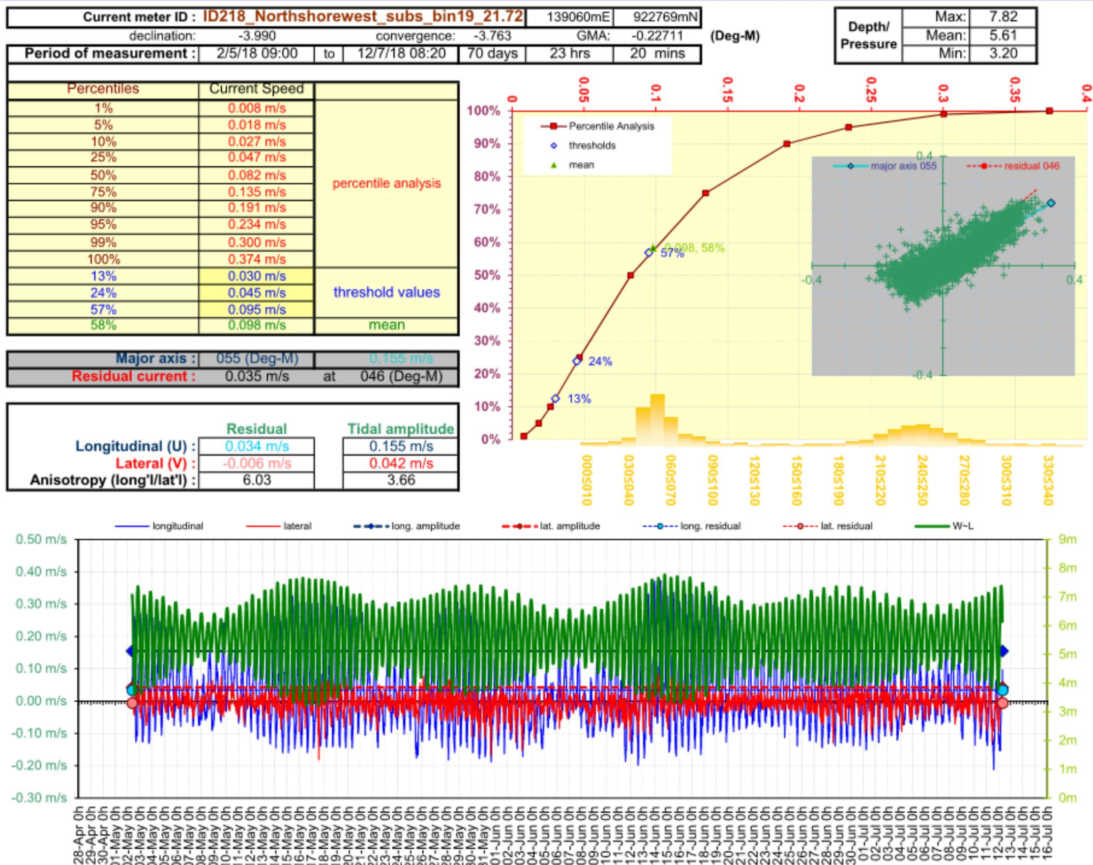
Figure 4. Current Data Summary Sheet for the surface current cell 19, 21.72 m from seabed, 2<sup>nd</sup> May to 12<sup>th</sup> July 2018 inclusive (ID218).
