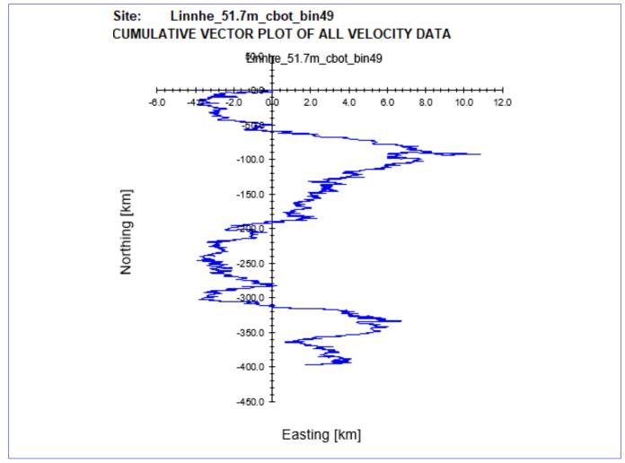
Figure 8. Cumulative Vector Plot of all velocity data from cage bottom cell for ID277.
