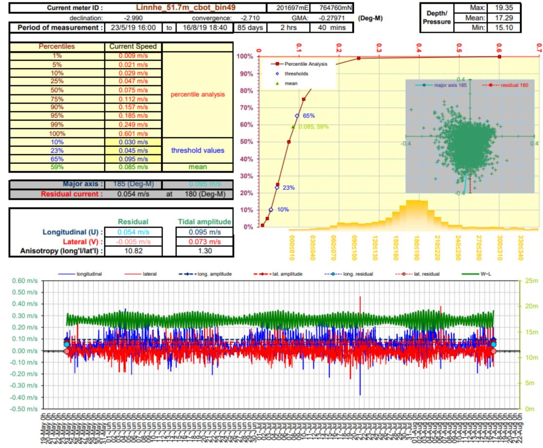
Figure 5. Current Data Summary Sheet for the cage bottom current cell 49, 51.71m from seabed, 23<sup>rd</sup> May to 16<sup>th</sup> August 2019 inclusive (ID277).
