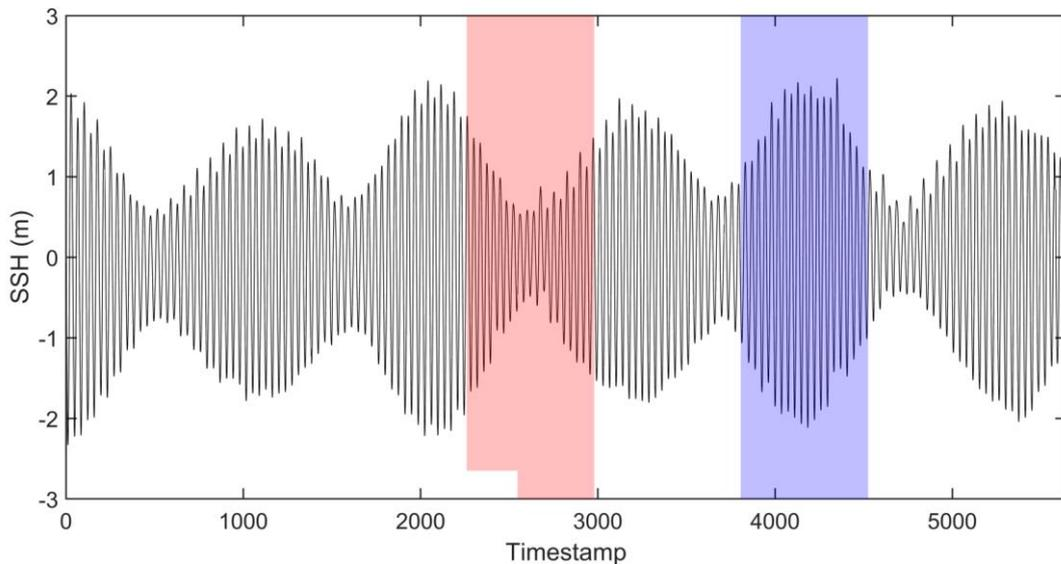
Figure 5. Sea surface height (SSH) at Hellisay from 13<sup>th</sup> August –30<sup>th</sup> October 2018 (ID239). Dispersion simulations were performed over periods of neap tides (red, start day 15<sup>th</sup> September 2018) and spring tides (blue, start day 6<sup>th</sup> October 2018)
