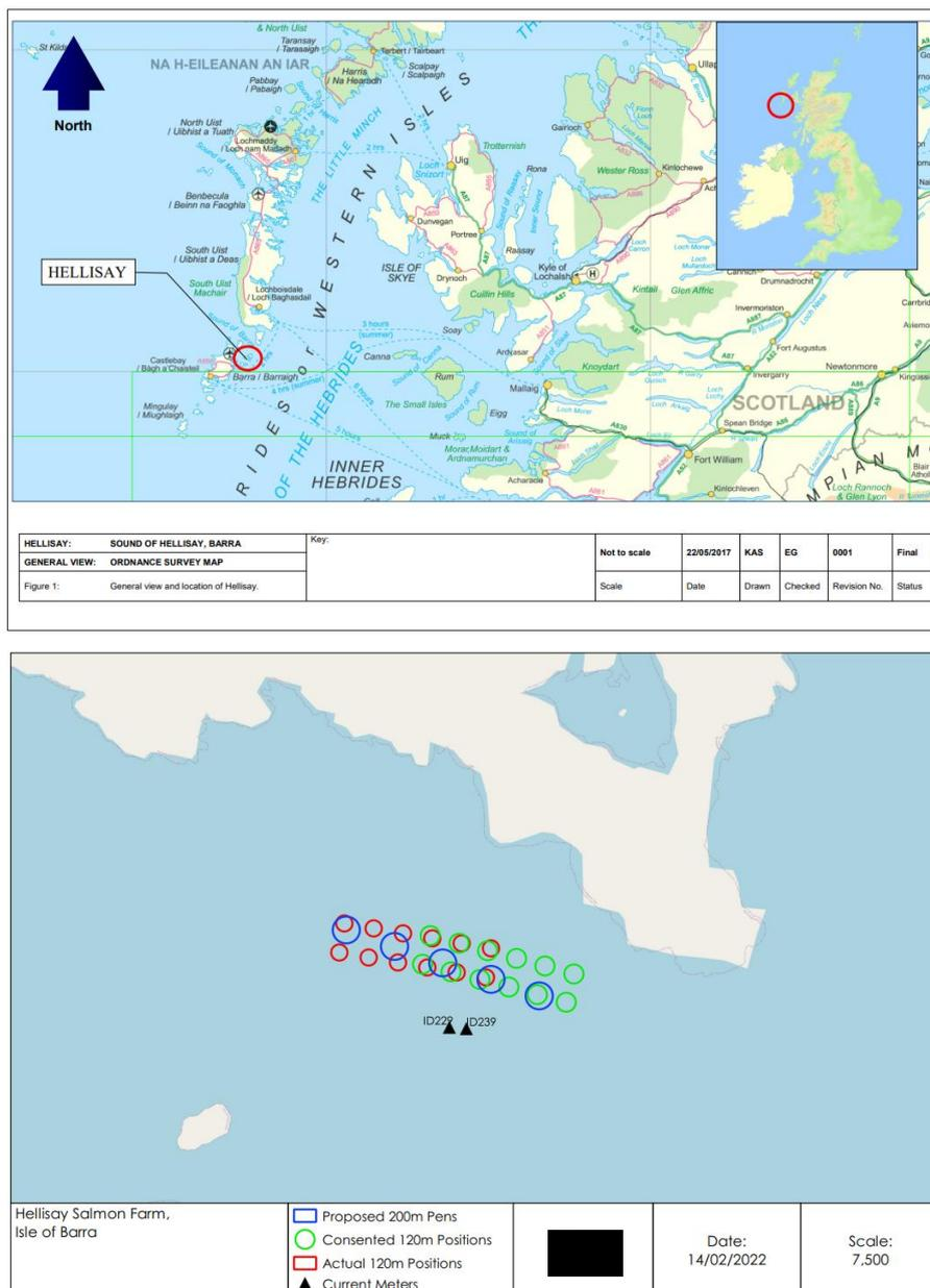
Figure 1. Location of Hellisay salmon farm (top) and the location of the ADCP deployments (▲) relative to the proposed pen positions (○).
