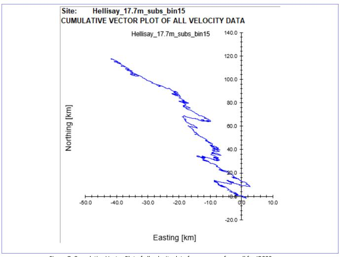
Figure 7. Cumulative Vector Plot of all velocity data from near surface cell for ID239.
