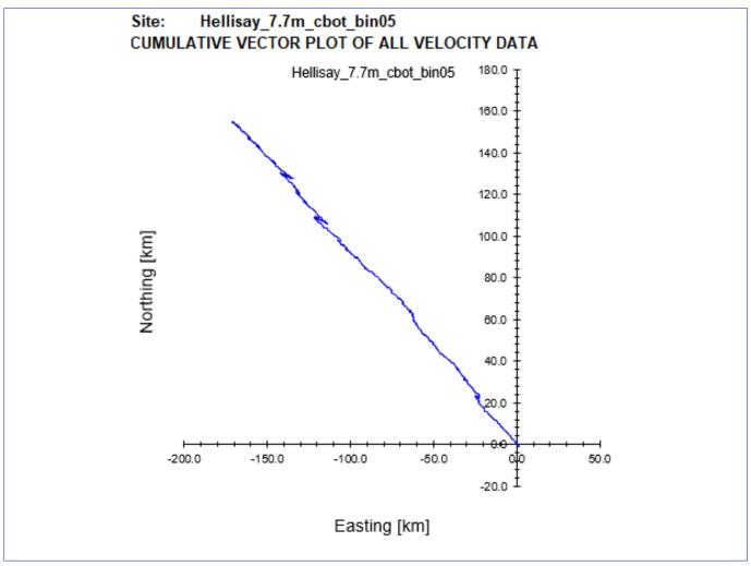
Figure 8. Cumulative Vector Plot of all velocity data from cage bottom cell for ID239.
