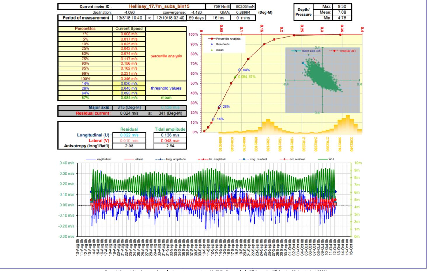
Figure 4. Current Data Summary Sheet for the surface current cell 15, 17.7m from seabed, 13th August to 12th October 2018 inclusive (ID239).
