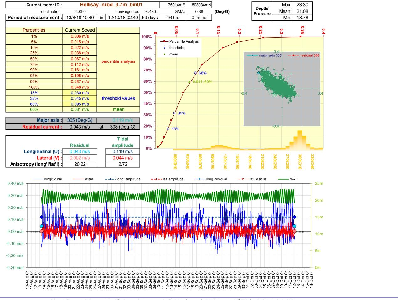
Figure 6. Current Data Summary Sheet for the near bottom current cell 1, 3.7m from seabed, 13th August to 12th October 2018 inclusive (ID239).
