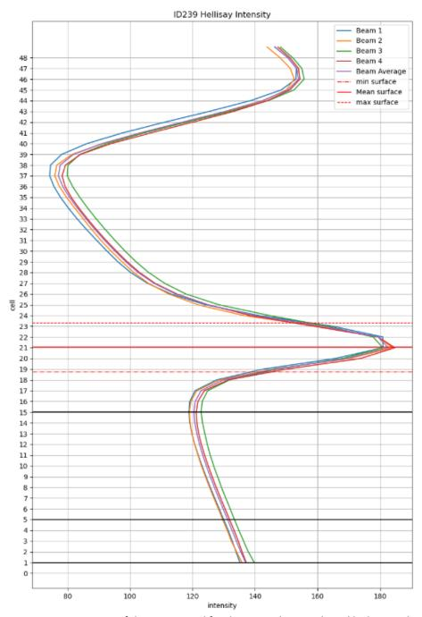
Figure 3. Mean intensity of the ADCP signal for the ID239 dataset plotted by bin number
