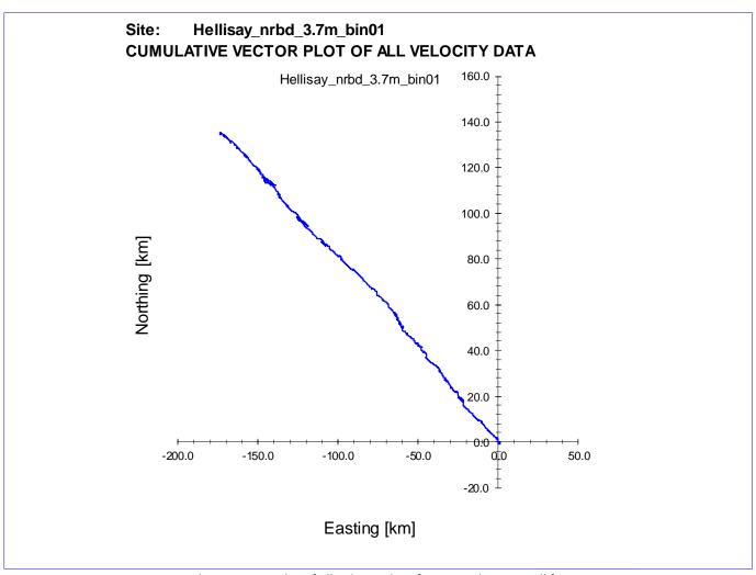
Figure 9. Cumulative Vector Plot of all velocity data from near bottom cell for ID239.
