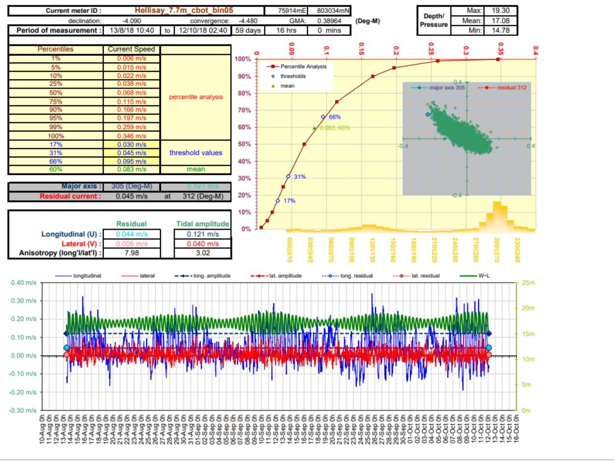
Figure 5. Current Data Summary Sheet for the cage bottom current cell 5, 7.7m from seabed, 13th August to 12th October 2018 inclusive (ID239).
