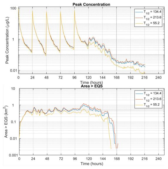
Figure 10. Time series of maximum concentration (top) and area exceeding the EQS (bottom) from the second set of model runs (Table 4). The model was run during neap tide with varying medicine half-life ( $T_{1/2}$ ). The MAC and area limit 72 hours after the final treatment (Time = 168 h) of 0.1 µg/L and 0.5 km<sup>2</sup> are indicated by the horizontal dashed lines.
