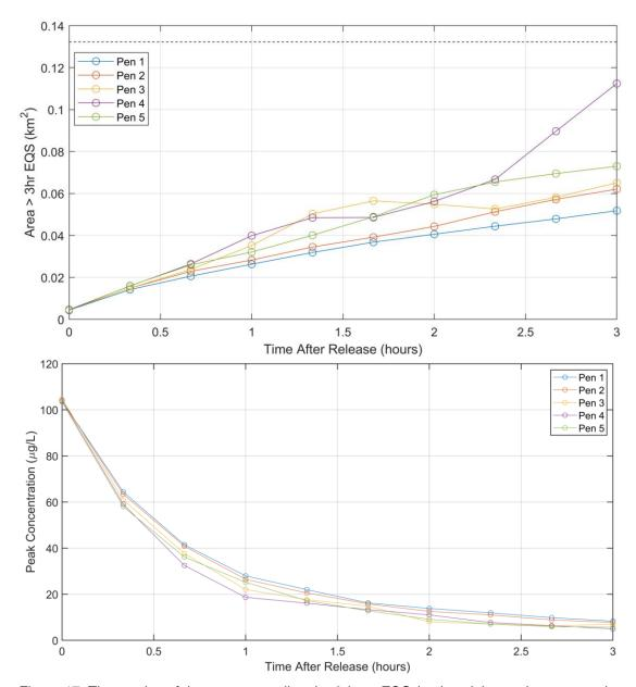
Figure 17. Time series of the area exceeding the 3-hour EQS (top) and the peak concentration (bottom) for each individual pen treatment during the 3 hours following release at spring tide. The 3-hour mixing zone area indicated (---).
