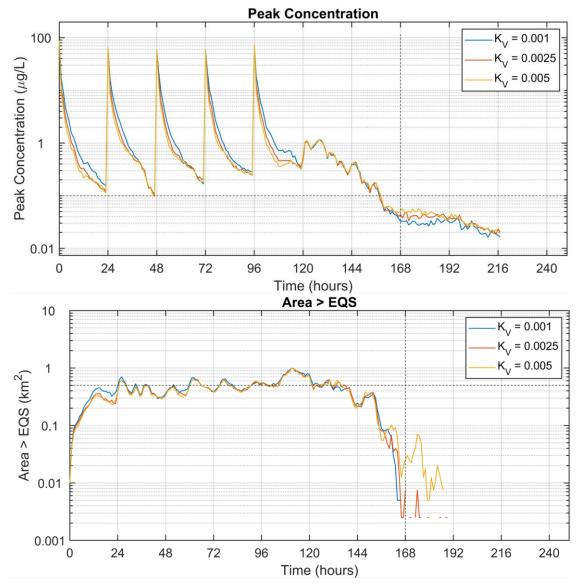
Figure 12. Time series of maximum concentration (top) and area exceeding the EQS (bottom) from the fourth set of model runs (Table 4). The model was run during neap tides with varying vertical diffusion coefficient  $K_V$  ( $m^2$  s<sup>-1</sup>). The MAC and area limit 72 hours after the final treatment (Time = 168 h) of 0.1 µg/L and 0.5 km² are indicated by the horizontal dashed lines.
