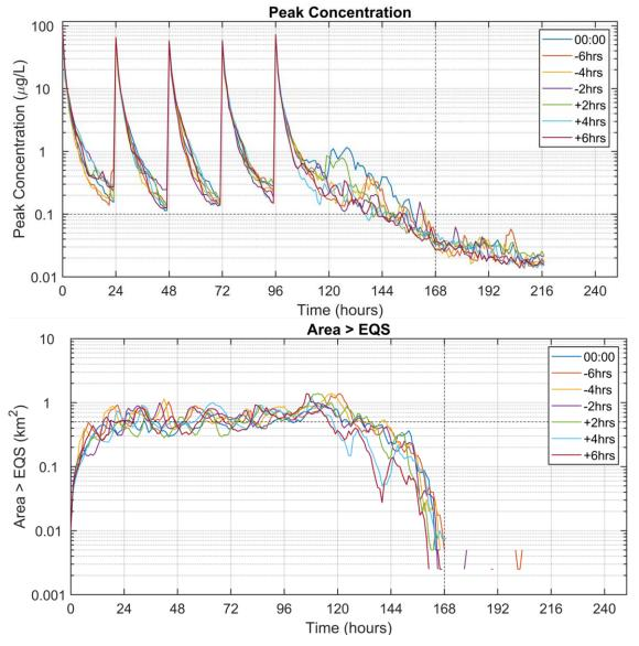
Figure 13. Time series of maximum concentration (top) and area exceeding the EQS (bottom) from the first set of model runs (Table 4). The model was run during neap tides with varying release times, relative to the baseline (Start = 0 h). The MAC and area limit 72 hours after the final treatment (Time = 168 h) of 0.1 µg/L and 0.5 km² are indicated by the horizontal dashed lines.
