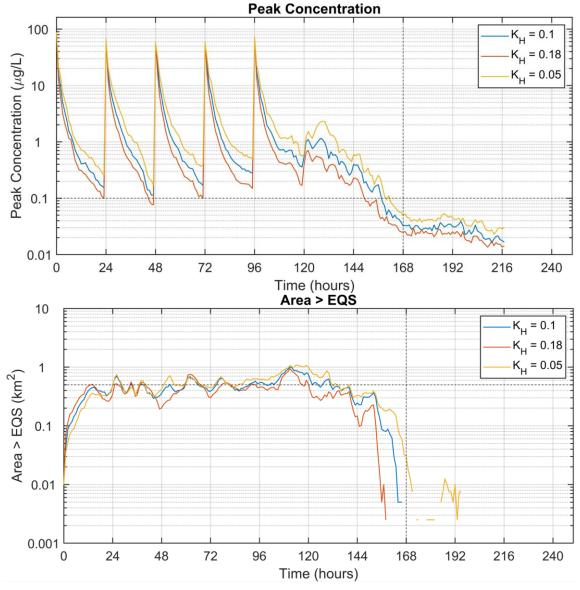
Figure 11. Time series of maximum concentration (top) and area exceeding the EQS (bottom) from the third set of model runs (Table 4). The model was run during neap tide with varying horizontal diffusion coefficient  $K_H$  ( $m^2$  s<sup>-1</sup>). The MAC and area limit 72 hours after the final treatment (Time = 168 h) of 0.1 µg/L and 0.5 km<sup>2</sup> are indicated by the horizontal dashed lines.
