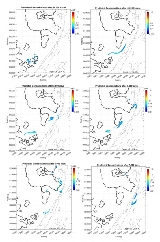
Figure 9. Predicted concentration fields for a dispersion simulation at neap tides after 24 hours (top left), 48 hours (top right), 72 hours (middle left), 96 hours (middle right), 120 hours (bottom left) and 168 hours (bottom right).
