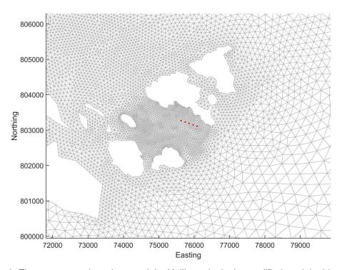
Figure 3. The unstructured mesh around the Hellisay site in the modified model grid, with the proposed pen locations indicated (o).
