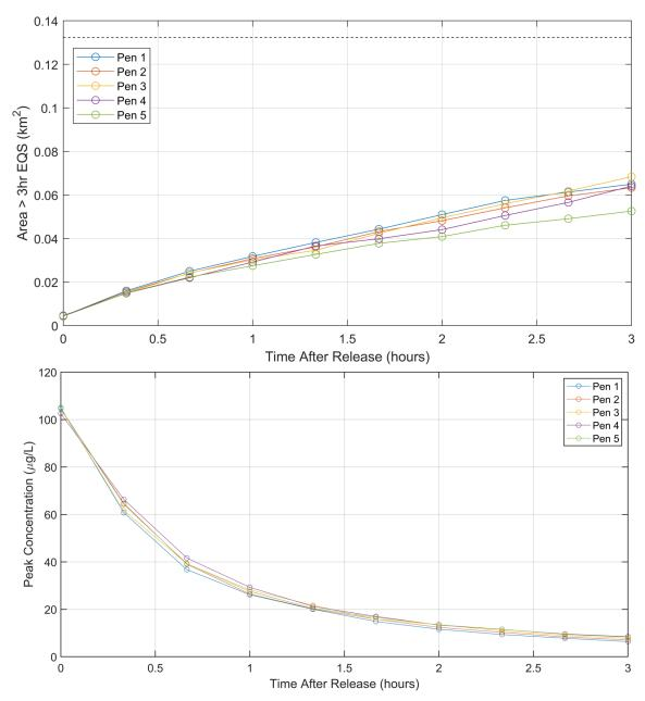
Figure 16. Time series of the area exceeding the 3-hour EQS (top) and the peak concentration (bottom) for each individual pen treatment during the 3 hours following release at neap tide. The 3-hour mixing zone area is indicated (---).
