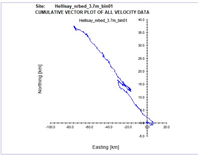
Figure 9. Cumulative Vector Plot of all velocity data from near bottom cell for ID229.
