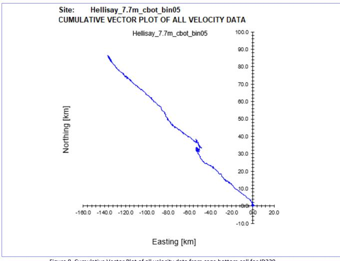
Figure 8. Cumulative Vector Plot of all velocity data from cage bottom cell for ID229.
