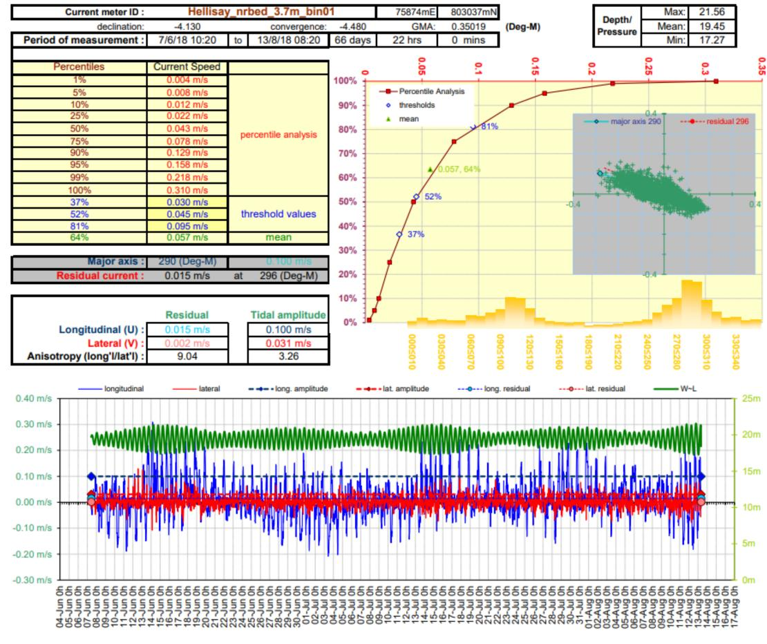
Figure 6. Current Data Summary Sheet for the near bottom current cell 1, 3.7m from seabed, 7<sup>th</sup> June to 13<sup>th</sup> August 2018 inclusive (ID229).
