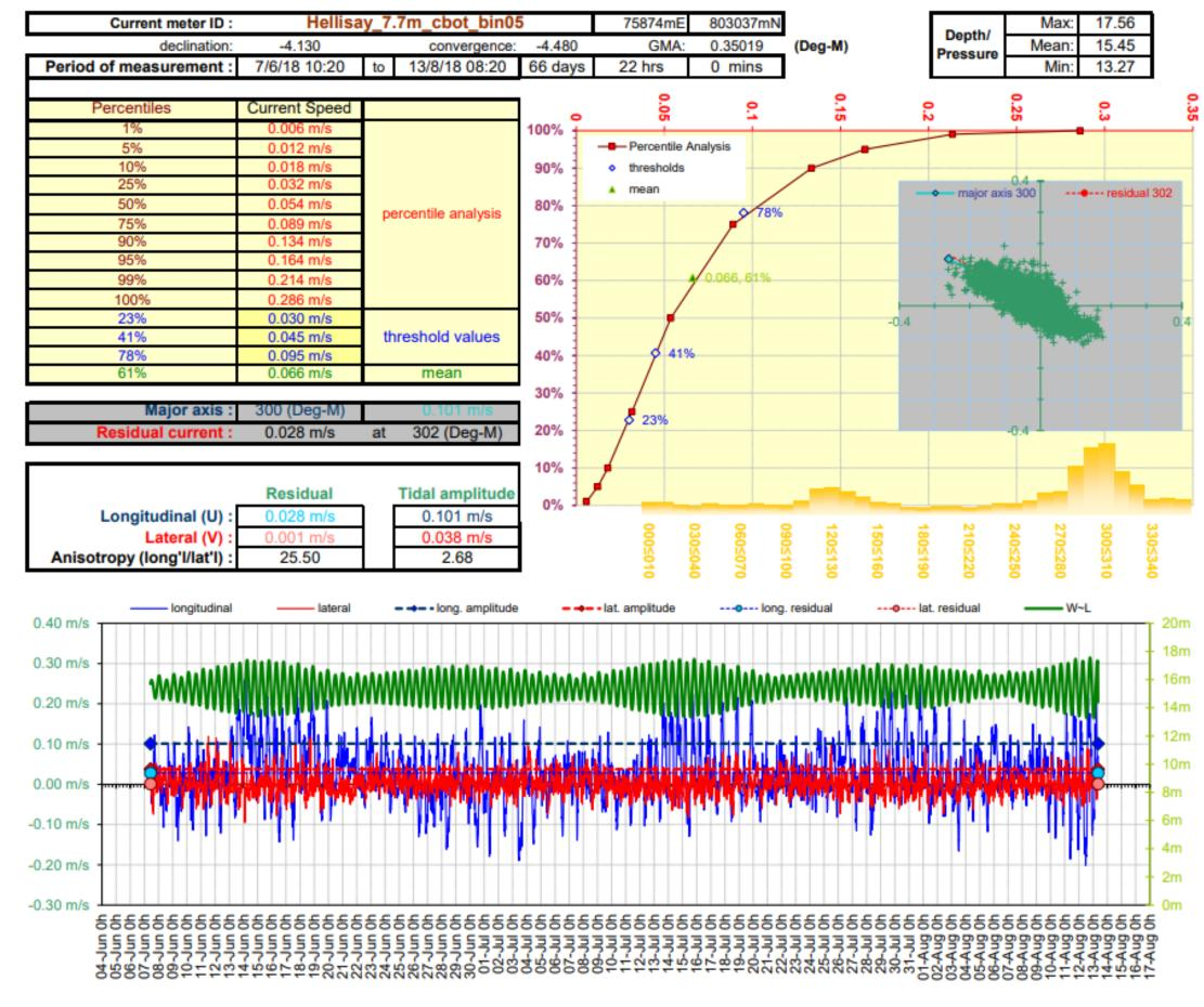
Figure 5. Current Data Summary Sheet for the cage bottom current cell 5, 7.7m from seabed, 7<sup>th</sup> June to 13<sup>th</sup> August 2018 inclusive (ID229).
