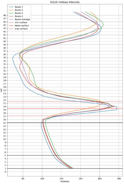
Figure 3. Mean intensity of the ADCP signal for the ID229 dataset plotted by bin number
