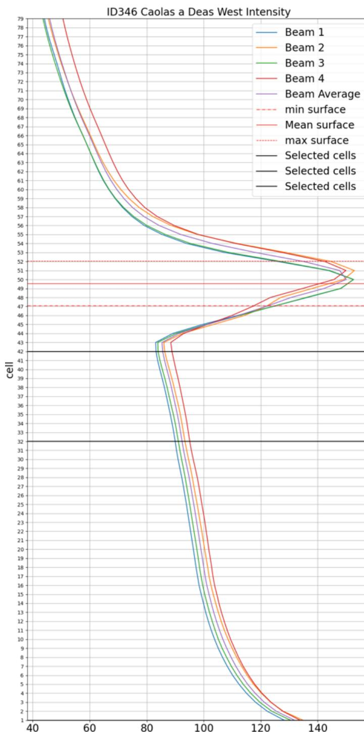
Figure 3. Mean intensity of the ADCP signal for the ID346 dataset plotted by bin number
