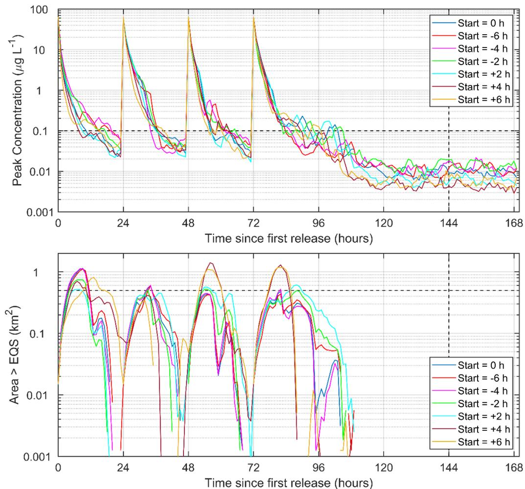
Figure 14. Time series of maximum concentration (top) and the area where concentrations exceeded the EQS (bottom) from the seventh set of model runs (Table 4). The model was run at spring tides with varying release times relative to the baseline (Start = 0 h). The MAC and area limit 72 hours after the final treatment (Time = 144 h) of  $0.1 \mu\text{g L}^{-1}$  and  $0.5 \text{km}^2$  are indicated by the horizontal dashed lines.
