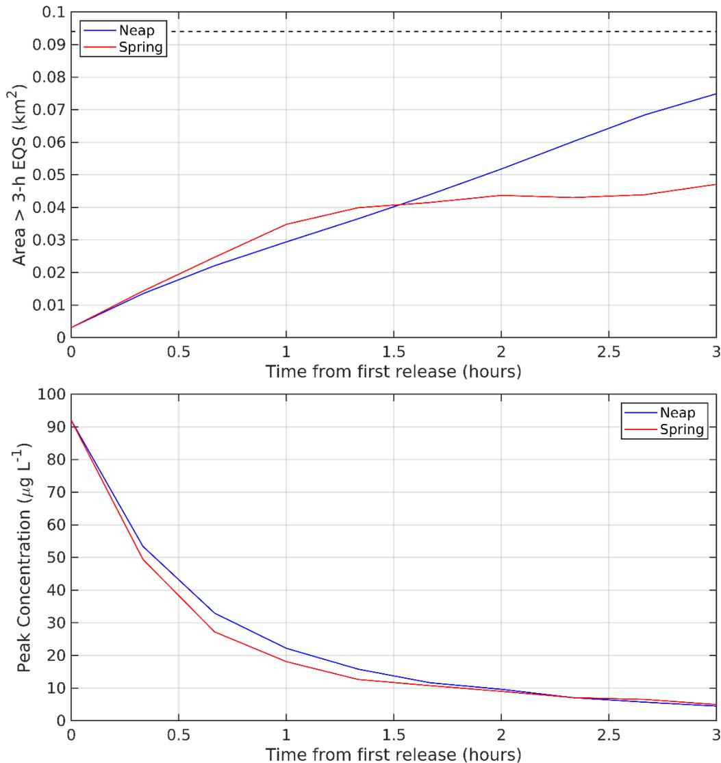
Figure 18. Time series of the area exceeding the 3-hour EQS (top) and peak concentrations (bottom) for a pen treatment during the three hours following release at spring and neap tides. The 3-hour mixing zone area is indicated (---).
