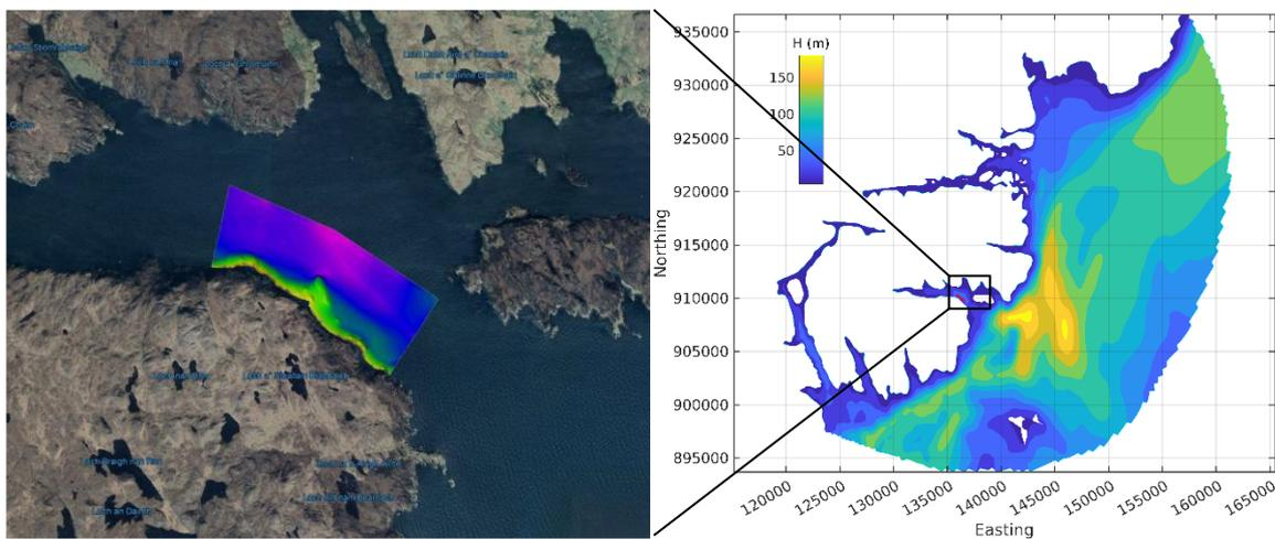
Figure 4. Multibeam survey of bathymetry around Caolas a Deas farm sites from December 2020 (left). Model water depths ( $H$ , m) in the model domain (right), incorporating the multibeam data. The proposed cage locations are indicated (●).
