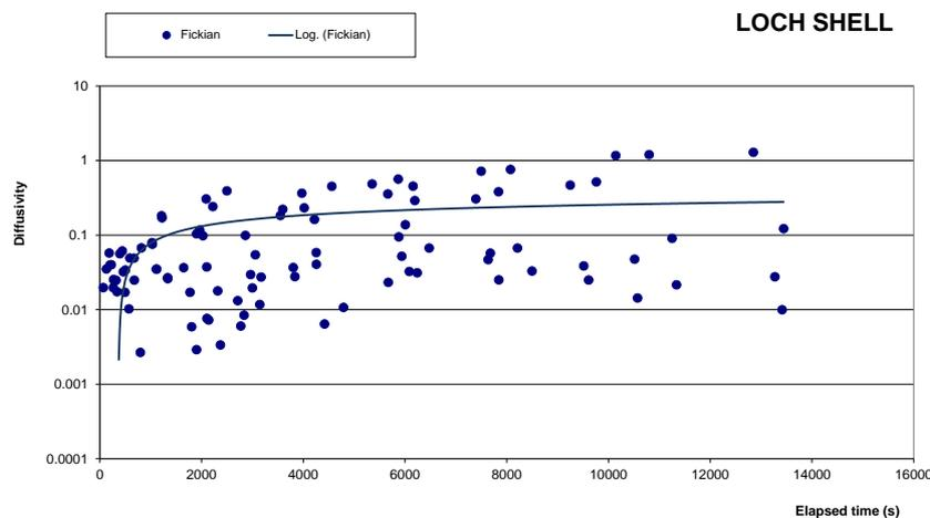
Figure 7. Estimated horizontal diffusivity ( $\text{m}^2 \text{ s}^{-1}$ ) from dye release experiments at Caolas a Deas, Loch Shell, on 23<sup>rd</sup> July 2020. The mean diffusivity was  $0.15 \text{ m}^2 \text{ s}^{-1}$ .
