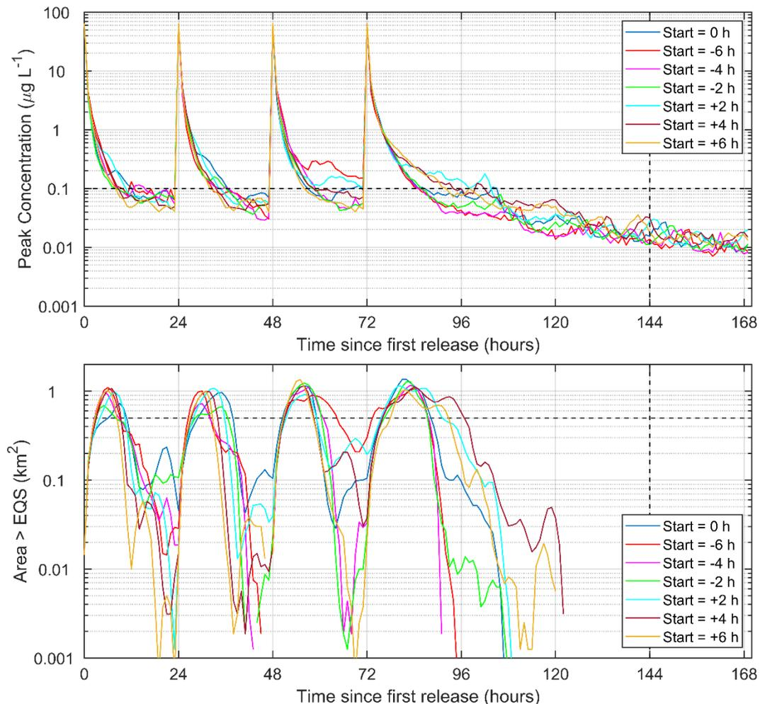
Figure 12. Time series of maximum concentration (top) and area exceeding the EQS (bottom) from the fourth set of model runs (Table 4). The model was run during neap tides with varying release times, relative to the baseline (Start = 0 h). The MAC and area limit 72 hours after the final treatment (Time = 144 h) of  $0.1 \mu\text{g L}^{-1}$  and  $0.5 \text{ km}^2$  are indicated by the horizontal dashed lines.
