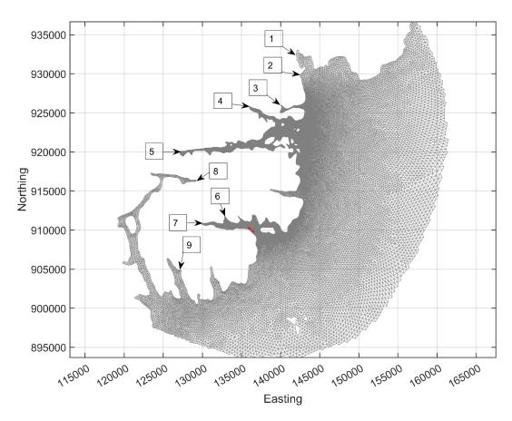
Figure 2. The model mesh and domain for the Outer Loch Shell modelling study. The proposed cage locations ( $\bullet$ ) are indicated, as are locations of freshwater discharge ( $\rightarrow$ ).
