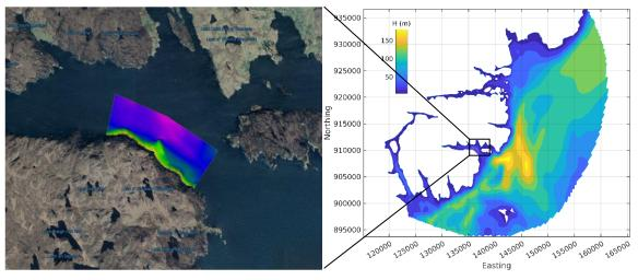
Figure 4. Multibeam survey of bathymetry around Caolas a Deas farm sites from December 2020 (left). Model water depths (H, m) in the model domain (right), incorporating the multibeam data. The proposed cage locations are indicated (•).
