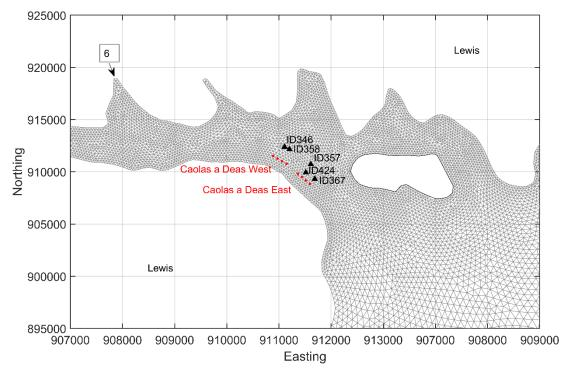
Figure 3. ADCP deployment locations ID346, ID357, ID358, ID367 and ID424 (▲) and locations of freshwater discharge (→) are also indicated.
