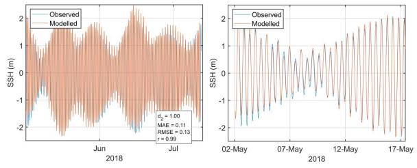
Figure 9. Comparison between observed and modelled sea surface height from May – July 2018 (ADCP deployment ID218) using model parameter values from Table 1. Both the full record (left) and a subset of 15 days (right) are shown. Observed data are in blue, model results in red.
