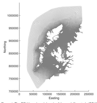
Figure 1. The ECLH mesh and domain of the modelling study (SSM)
