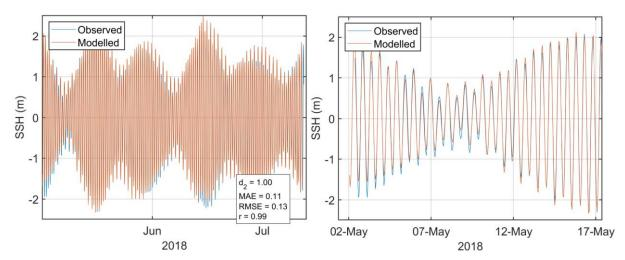
Figure 13. Comparison between observed and modelled sea surface height from May – July 2018 (ADCP deployment ID219) using model parameter values from Table 1. Both the full record (left) and a subset of 15 days (right) are shown. Observed data are in blue, model results in red.
