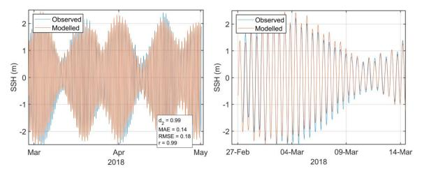
Figure 5. Comparison between observed and modelled sea surface height from February – May 2018 (ADCP deployment ID194) using model parameter values from Table 1. Both the full record (left) and a subset of 15 days (right) are shown. Observed data are in blue, model results in red.
