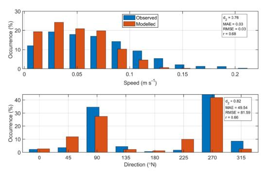
Figure 16. Histograms of observed and modelled current speed (top) and direction (bottom) at the ADCP location from May – July 2018 (ID219). Observed data are in blue, model results in red.
