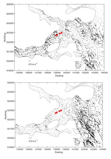
Figure 17. Modelled flood (top) and ebb (bottom) surface current vectors during spring tides. For clarity, only every 10<sup>th</sup> vector is shown.
