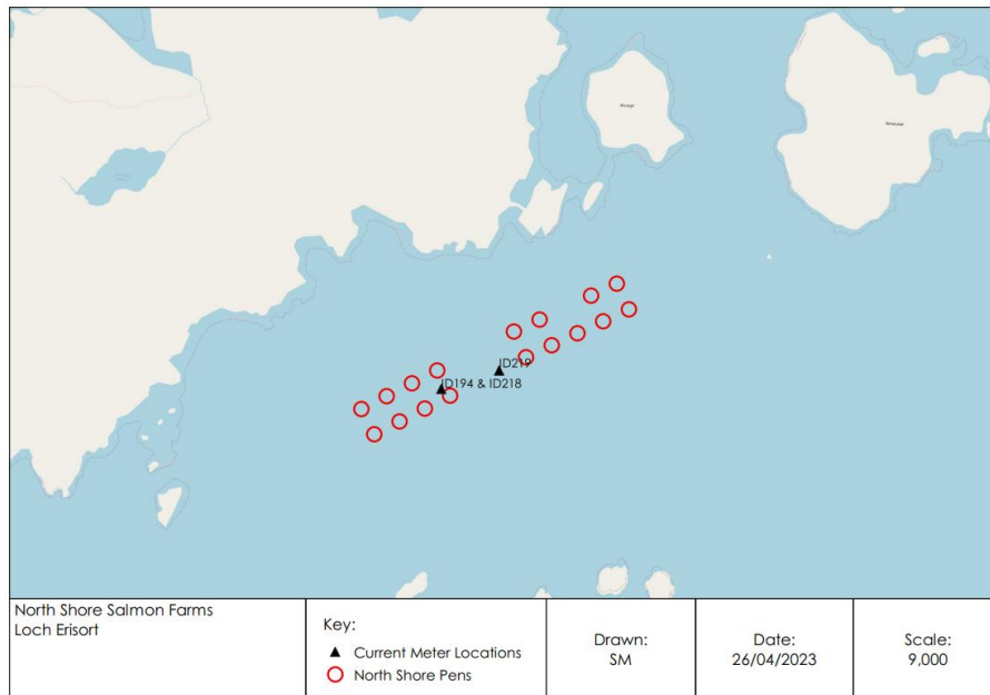
Figure 1. Location of the two salmon farms, North Shore East (right group) and the neighbouring site North Shore West (left group) and the location of the ADCP deployments (▲) relative to the pen positions (○).
