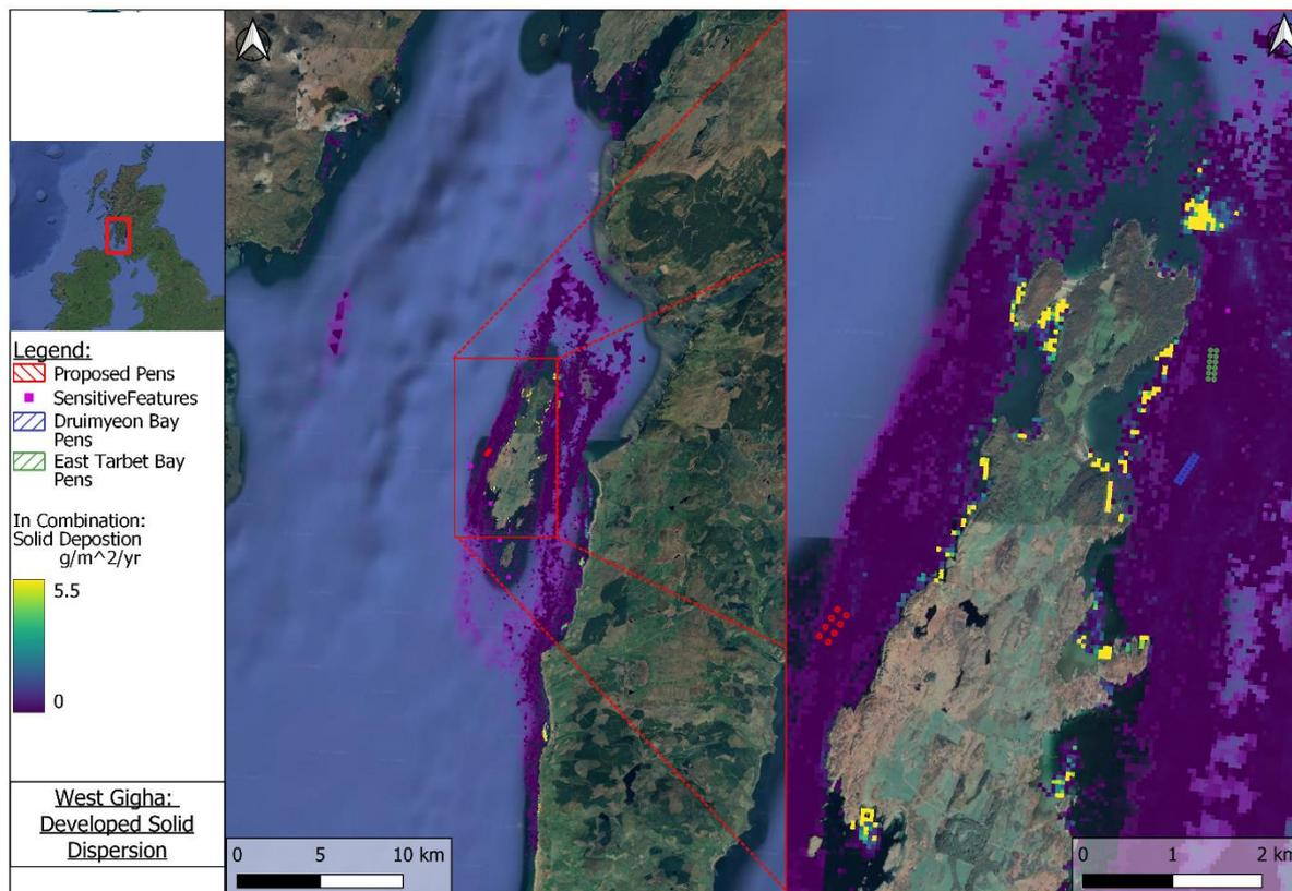
**Figure 4.3: In combination Solids deposition [g/m<sup>2</sup>/year] from West Gigha, Druimyeon Bay and East Tarbert Bay.** Blue and green circles indicate the pen locations at existing farms, Druimyeon Bay and East Tarbert Bay. Red circles indicate the proposed pen locations at the West Gigha farm site. pink dots indicate the location of identified Priority Marine Features.
