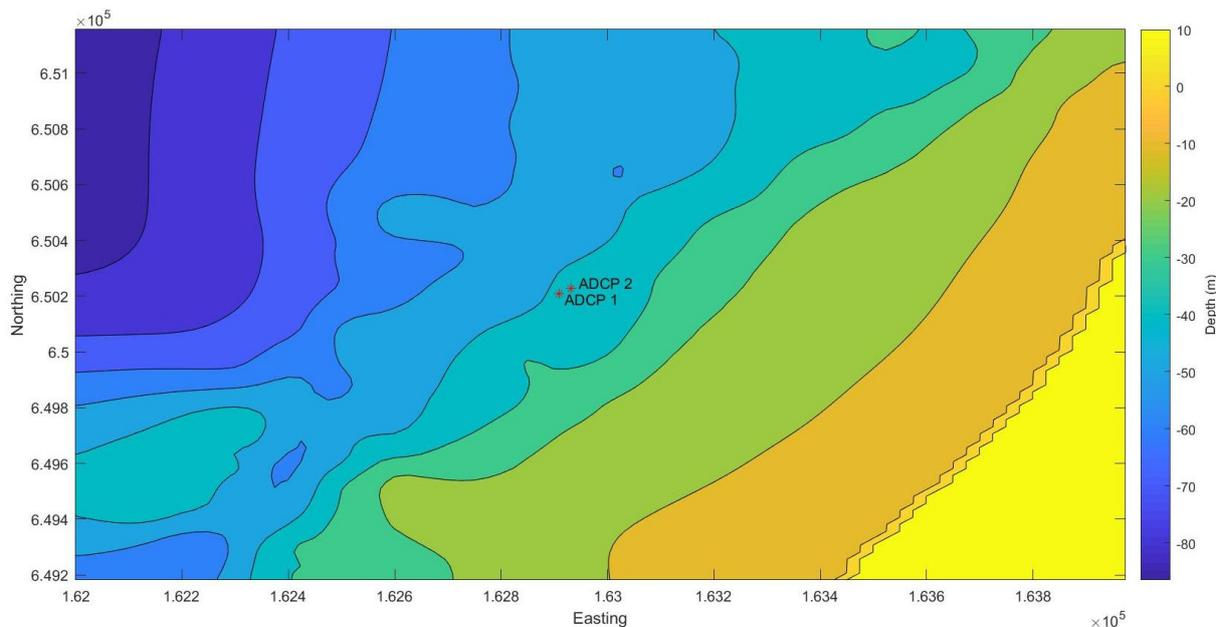
**Figure 4.1. Representation of bathymetry in a 2 x 2 km grid around the proposed West Gigha site. The two current meter locations are shown (ADCP1 and ADCP2).**
