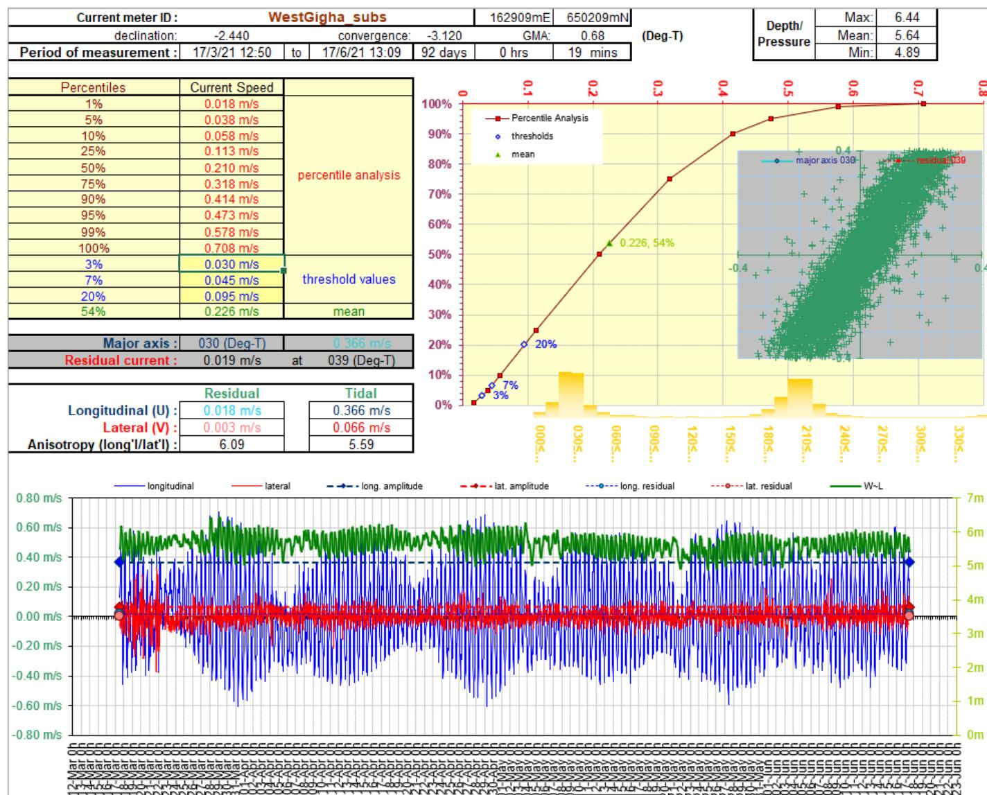
Figure 7.7. HG analysis summary of the sub-surface cell for West Gigha 92 days.
