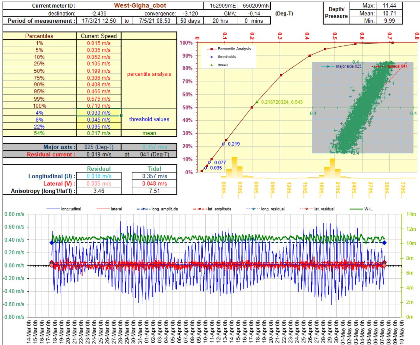
Figure 7.2. HG analysis summary of the cage-bottom cell for West Gigha 1<sup>st</sup> deployment.
