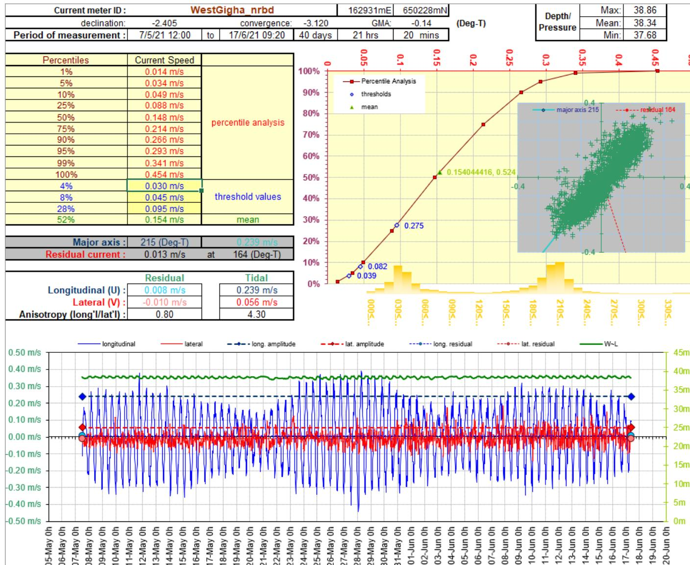
Figure 7.6. HG analysis summary of the near-bed cell for West Gigha 2<sup>nd</sup> deployment.
