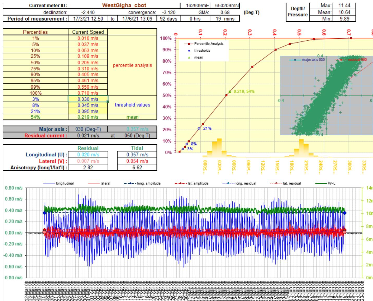
Figure 7.8. HG analysis summary of the cage-bottom cell for West Gigha 92 days.
