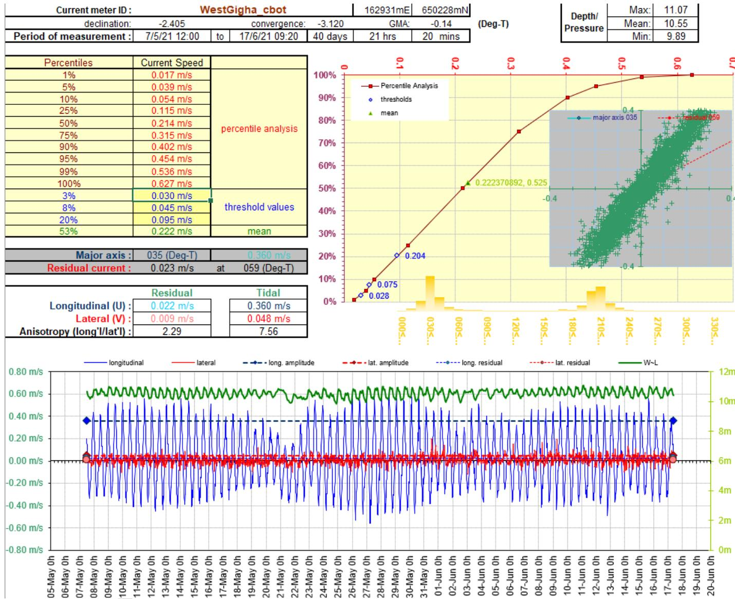
Figure 7.5. HG analysis summary of the cage-bottom cell for West Gigha 2<sup>nd</sup> deployment.
