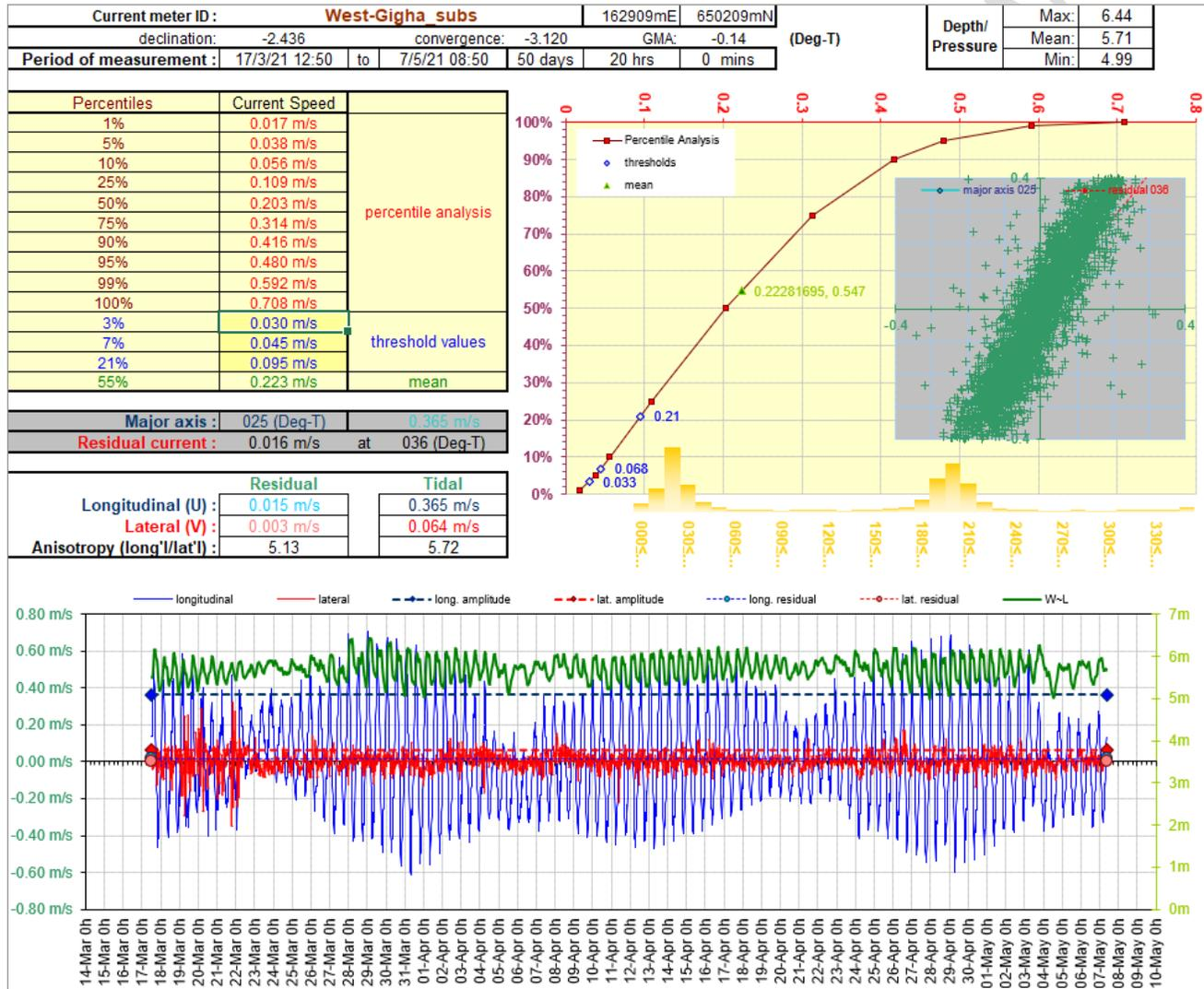
Figure 7.1. HG analysis summary of the sub-surface cell for West Gigha 1<sup>st</sup> deployment.
