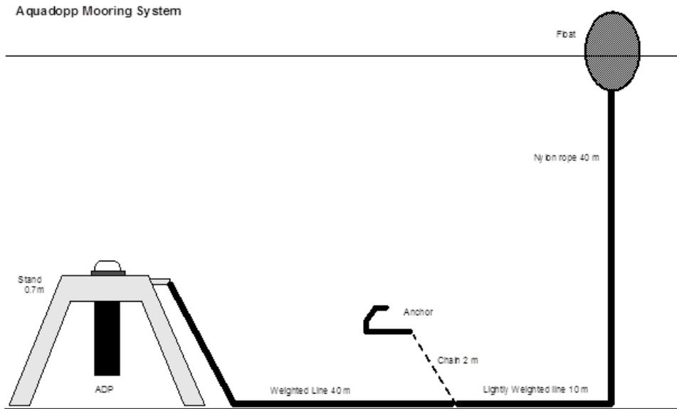
Figure 3.1: Example ADCP mooring system used during deployment.
