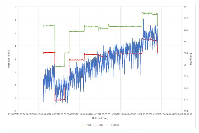
Figure 5.2: Pitch, Roll and Heading data for duration of ADCP deployment.
