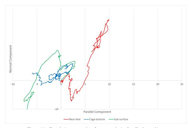
Figure 6.1: Cumulative vector plot of current velocity for all relevant bins.
