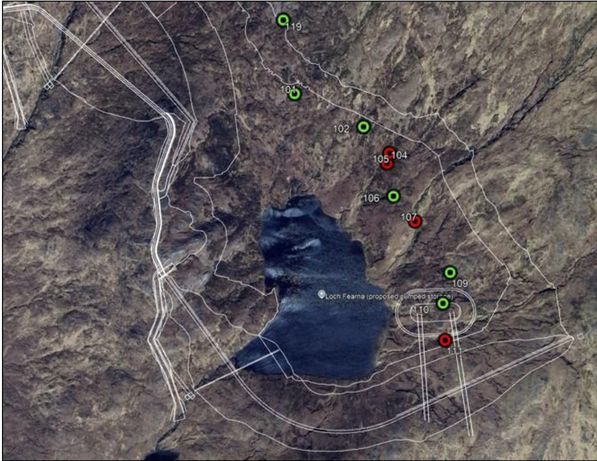
Figure 2. Extents of southern reservoir shoreline survey, with locations of identified intercepted streams (red = Type A alluvial channels, green = Type B colluvial channels).
