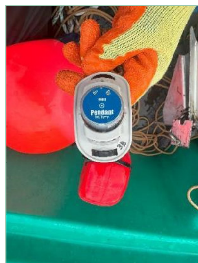
Solinst Levellogger and Hobo MX2200 Pendant instruments as deployed (Locations 4cA and 3b respectively)
