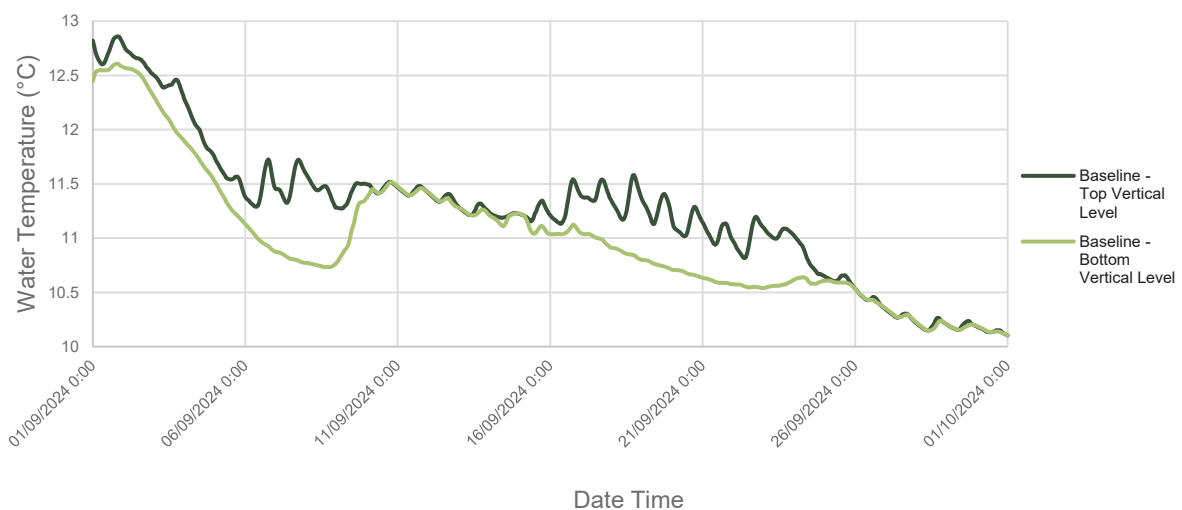
Figure 3-5: Vertical Temperature Profile at Dam Outtake (Baseline 2024)
