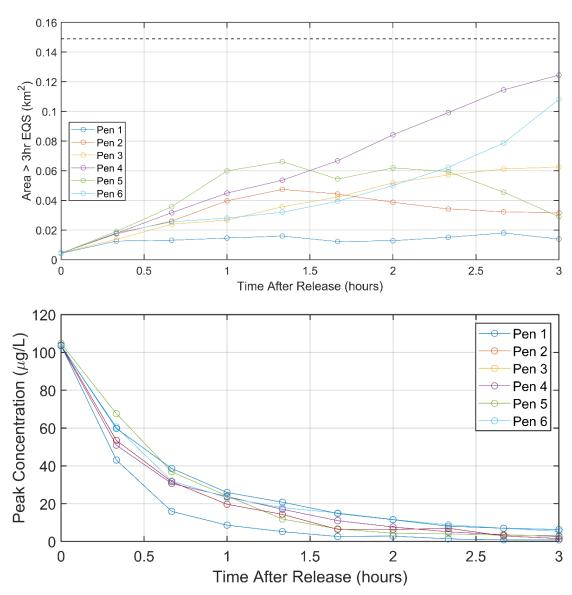
Figure 14. Time series of the area exceeding the 3-hour EQS (top) and the peak concentration (bottom) for each individual pen treatment during the 3 hours following release at neap tide. The 3-hour mixing zone area is indicated (---).
