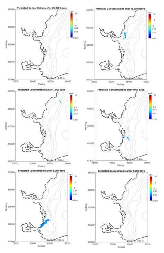
Figure 9. Predicted concentration fields for a dispersion simulation at neap tides after 24 hours (top left), 48 hours (top right), 72 hours (middle left), 96 hours (middle right), 120 hours (bottom left) and 192 hours (bottom right).
