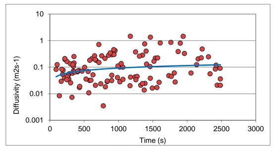
Figure 7. Estimated horizontal diffusivity (m<sup>2</sup> s<sup>-1</sup>) from dye release experiments at Stulaigh on 25<sup>th</sup> April 2017. The mean diffusivity was 0.18 m<sup>2</sup> s<sup>-1</sup>.
