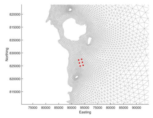
Figure 3. The unstructured mesh around the proposed Stulaigh South site in the modified model grid, with the proposed pen locations indicated (o).
