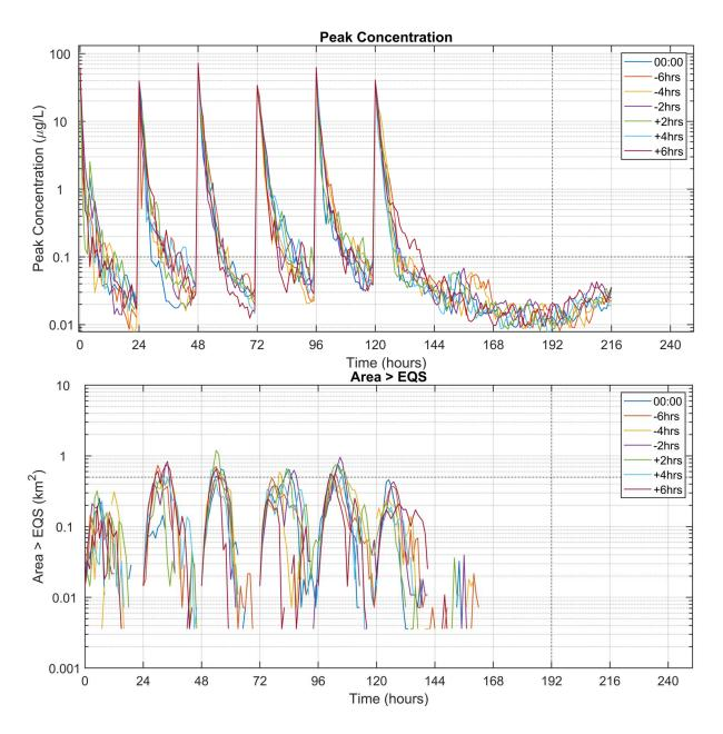
Figure 11. Time series of maximum concentration (top) and area exceeding the EQS (bottom) from the first set of model runs (Table 4). The model was run during neap tides with varying release times, relative to the baseline (Start = 0 h). The MAC and area limit 72 hours after the final treatment (Time = 192 h) of 0.1 µg/L and 0.5 km² are indicated by the horizontal dashed lines.
