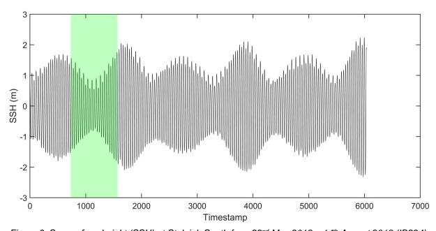
Figure 6. Sea surface height (SSH) at Stulaigh South from 22<sup>nd</sup> May 2018 – 14<sup>th</sup> August 2018 (ID224). Dispersion simulations were performed over periods of neap tides (green, start day 3<sup>rd</sup> June 2018).
