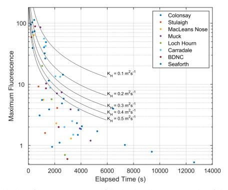
Figure 8. Maximum fluorescence measured following dye releases at a number of Mowi sites in Scotland. The black lines indicate the rate at which the maximum concentration would fall at different horizontal diffusivities.
