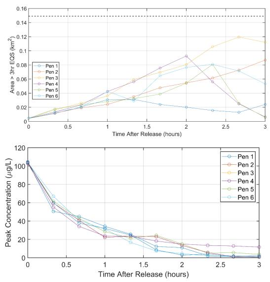
Figure 15. Time series of the area exceeding the 3-hour EQS (top) and the peak concentration (bottom) for each individual pen treatment during the 3 hours following release at spring tide. The 3-hour mixing zone area indicated (---).
