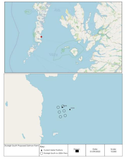
Figure 1. Site location (top) and layout (bottom) and of the proposed salmon farm off South Uist. The current meter deployment locations are marked by the black triangles.
