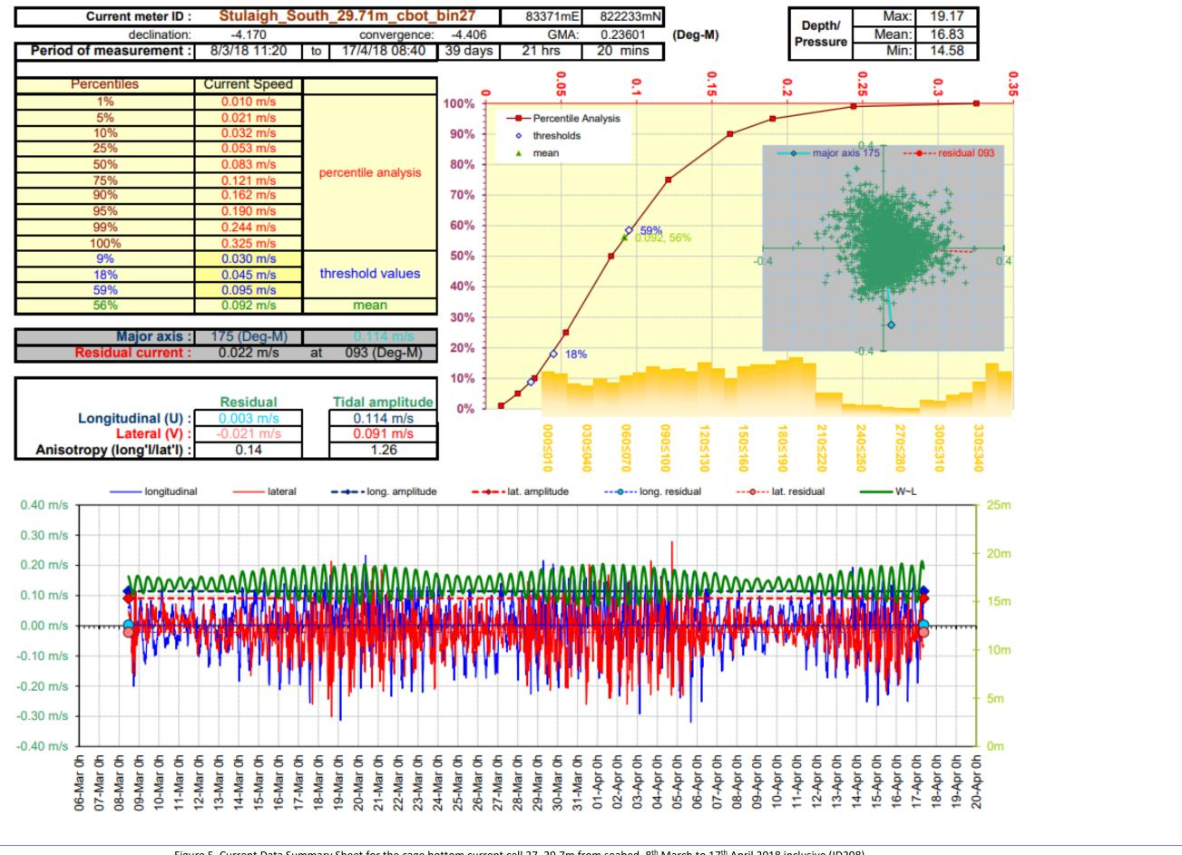
Figure 5. Current Data Summary Sheet for the cage bottom current cell 27, 29.7m from seabed, 8th March to 17th April 2018 inclusive (ID208).
