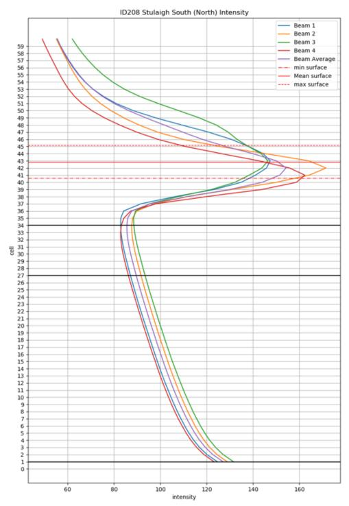
Figure 3. Mean intensity of the ADCP signal for the ID208 dataset plotted by bin number
