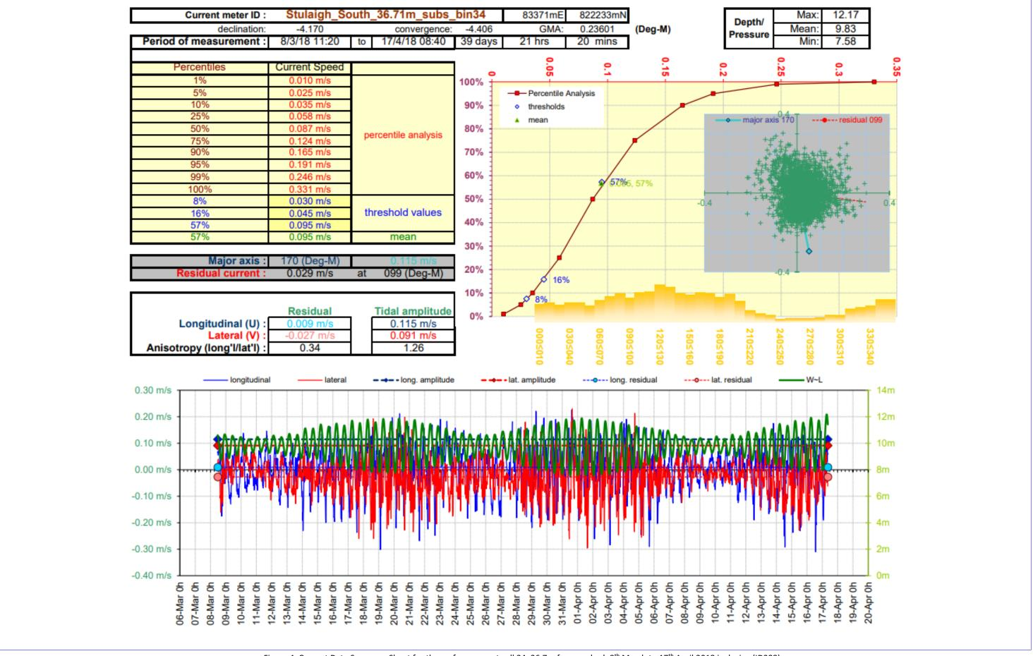
Figure 4. Current Data Summary Sheet for the surface current cell 34, 36.7m from seabed, 8th March to 17th April 2018 inclusive (ID208).
