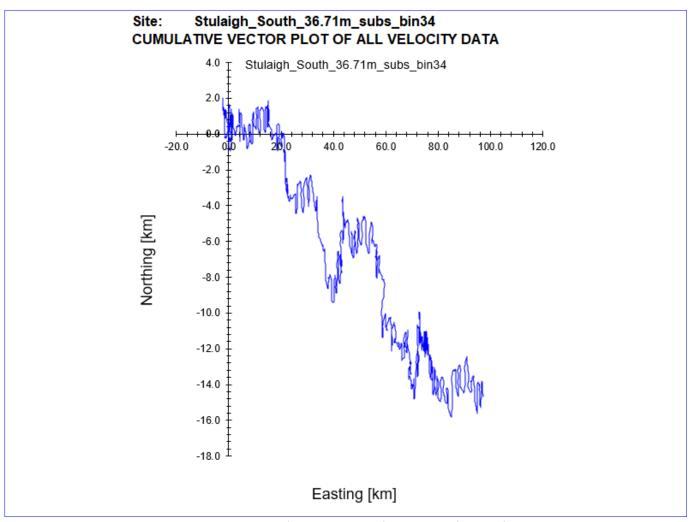
Figure 7. Cumulative Vector Plot of all velocity data from near surface cell for ID208.
