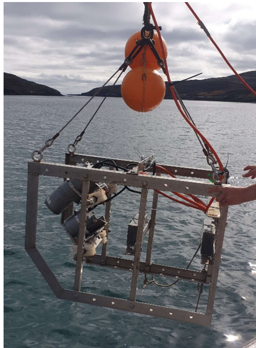
Figure 6.3 Drop-Down Video (DDV) System
