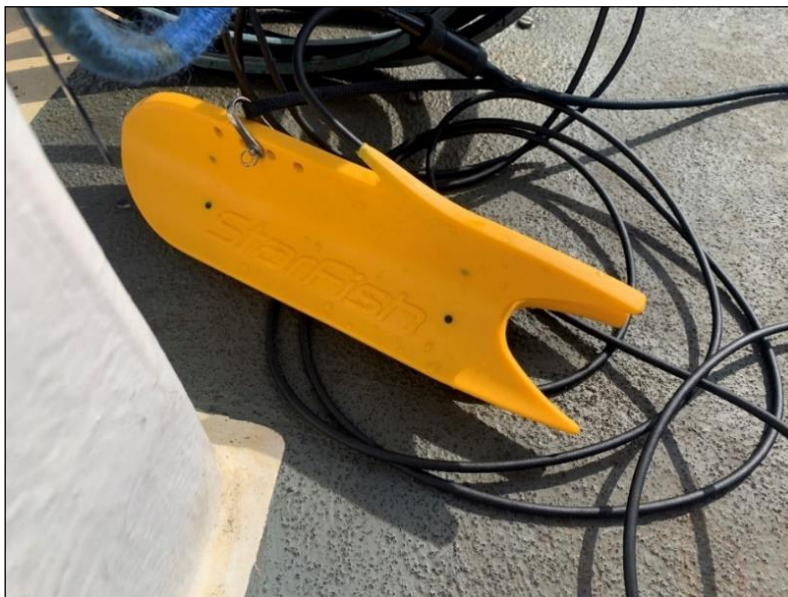
Figure 2.1 Blueprint Subsea StarFish 452F Side Scan Sonar
