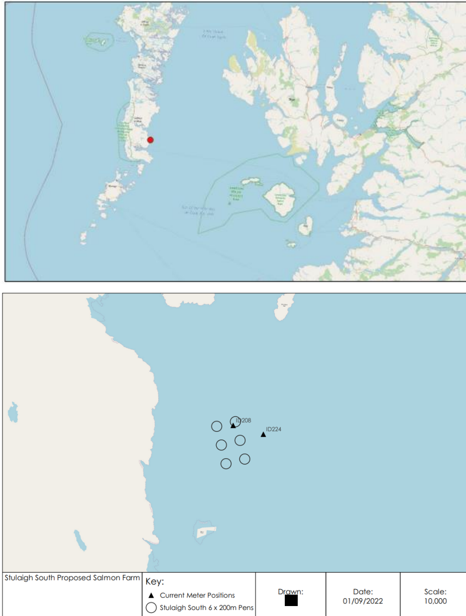
Figure 1. Location of the proposed Stulaigh South salmon farm (top) and the location of the ADCP deployments ID208 and ID224 (both from 2018) (▲) relative to the proposed pen positions (●).
