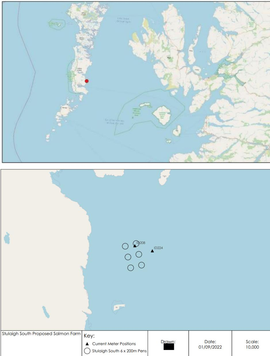
Figure 1. Location of the proposed Stulaigh South salmon farm (top) and the location of the ADCP deployments ID208 and ID224 (▲) relative to the proposed pen positions (○).
