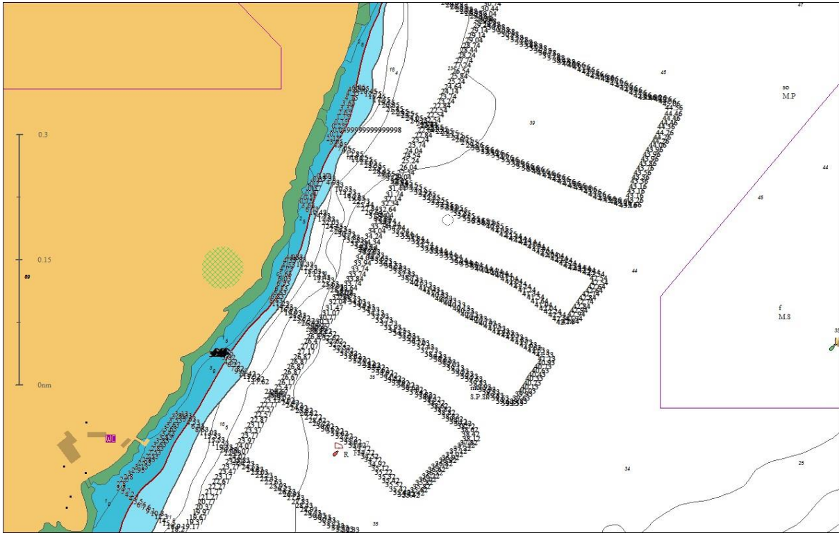
Figure 9.1: Cumbrae depth survey results plotted on Seapro
