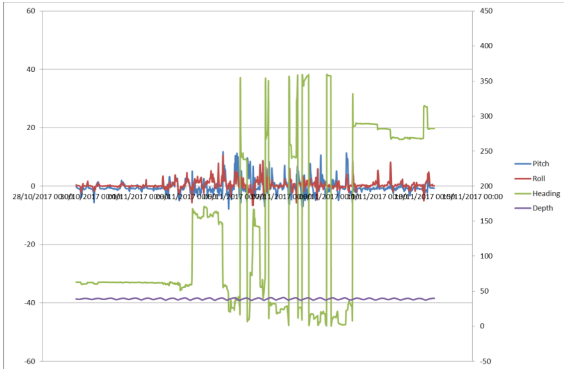
Figure 8.28: Heading, Depth, Pitch and Roll over the 15 days analysed
