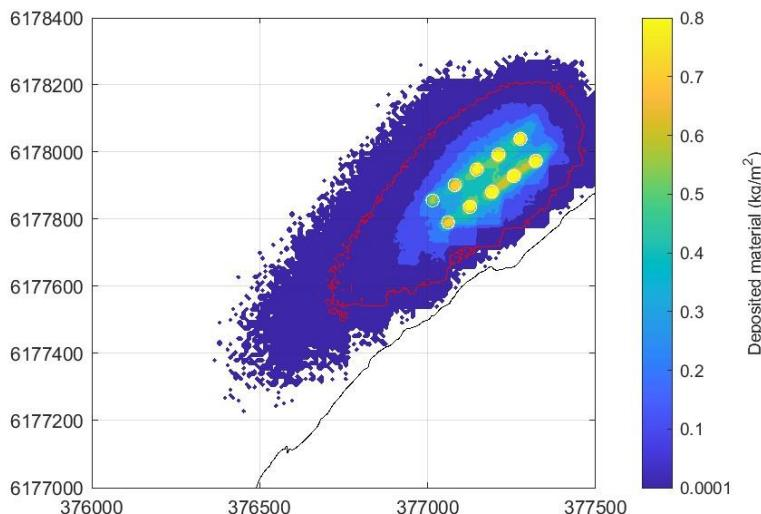
Figure 3.4 Deposited material at Little Cumbrae after 21-days – No wind applied. The red contour depicts the predicted 20g contour.
