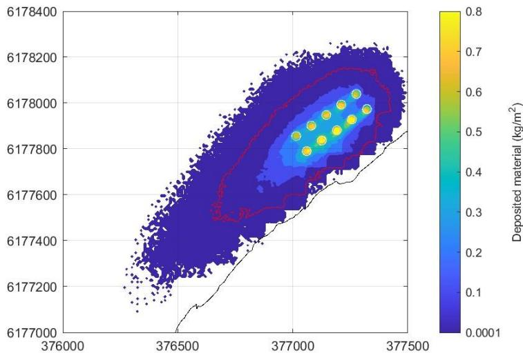
Figure 3.3 Deposited material at Little Cumbrae after 21-days - Wind applied. The red contour depicts the predicted 20g contour.
