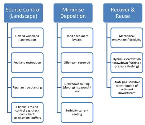
Figure 5-2: Indicative framework & example options for sediment management
