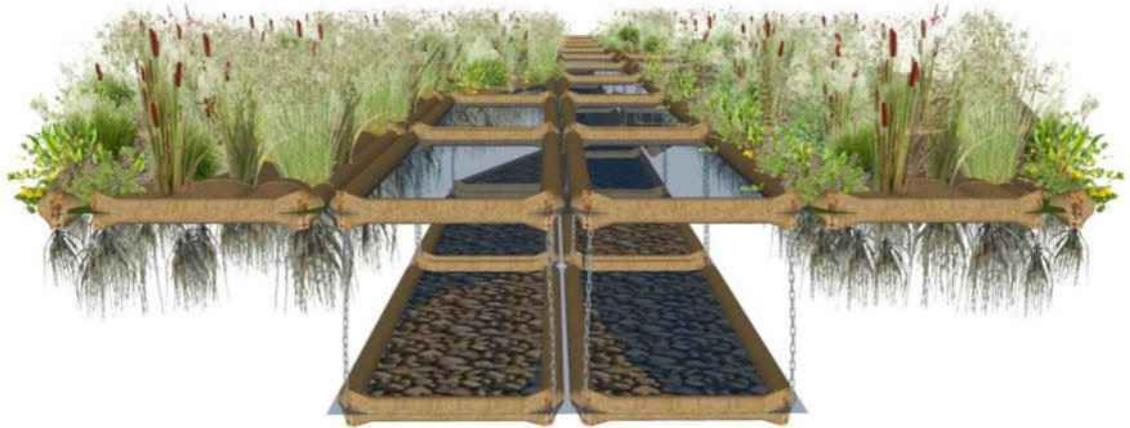
Figure 4. Potential Two-Tier Design with floating macrophyte beds and spawning substrate suspended below (Image Provided by Biomatrix)
