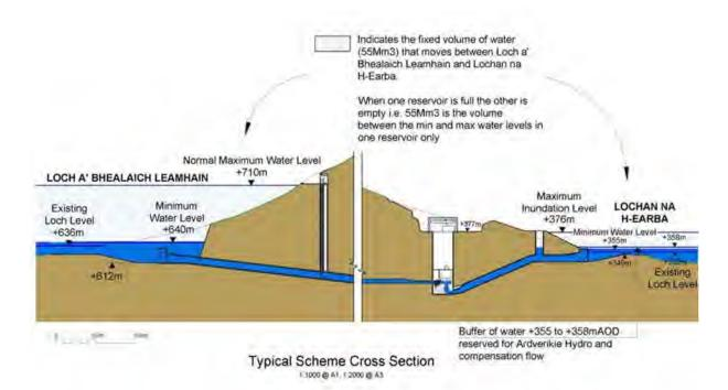
Plate 4-2 Cross Section through Upper and Lower Reservoirs
