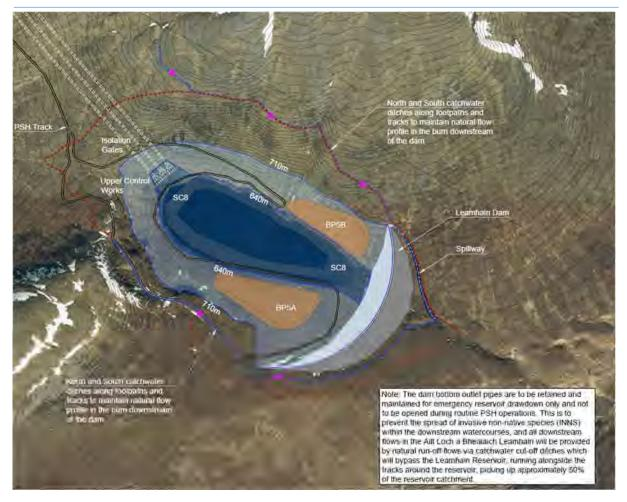
Figure 1 Extract from Figure 2.4 showing layout of channels to isolate catchment from reservoir
