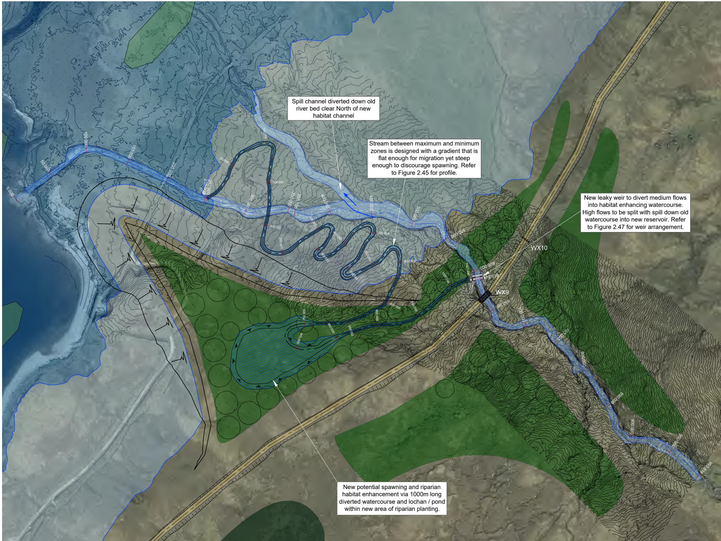
Spill channel diverted down old river bed clear North of new habitat channel
