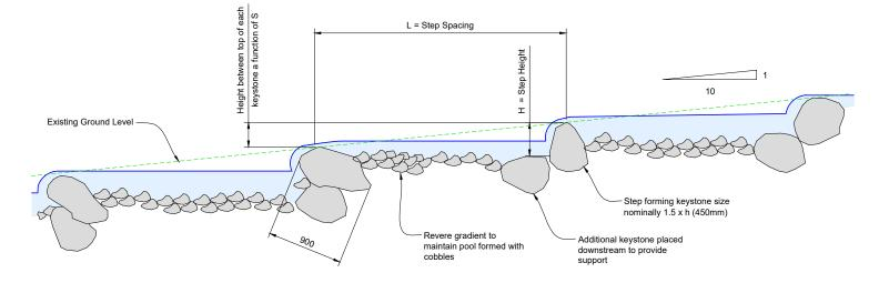
Typical Cascade Detail Pitridh Aqueduct Overflow and Leamhain Catchwater Ditch and Moy Spillway Channel 1:50 @ A3
