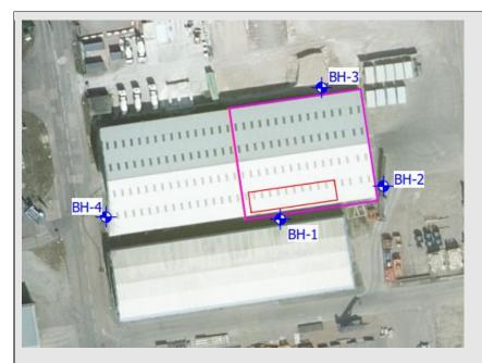
BH1 and BH2 were installed through low permeability deposits to bedrock thereby creating potential migration pathway to bedrock and the applicant was required to decommission, replace and resample these wells.
