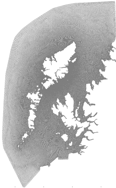
Figure 1. The mesh and domain of the East Coast of Lewis and Harris (ECLH) sub-model of the Scottish Shelf Model (Marine Scotland, 2016).
