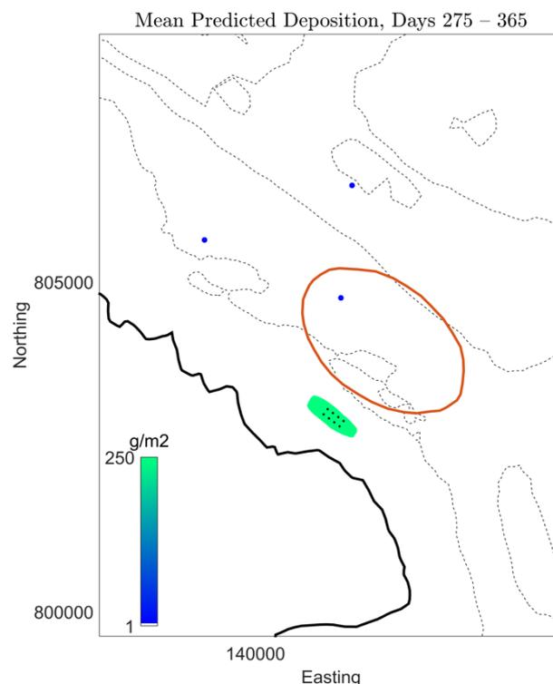
Figure 13. Identified PMF locations and the deposition footprint (shaded in green) predicted by marine modelling for the proposed new layout and biomass at the Rum site. Locations of the Tall Sea Pen PMFs (●) and Burrowed Mud PMF (red oval) are indicated.
