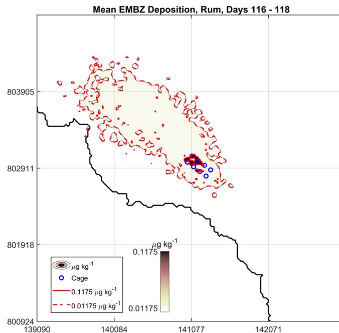
Figure 9: Predicted mean Emamectin Benzoate deposition over days 116-118 for the proposed 8 x 160m pens at Rum following a consented treatment of 12g.
