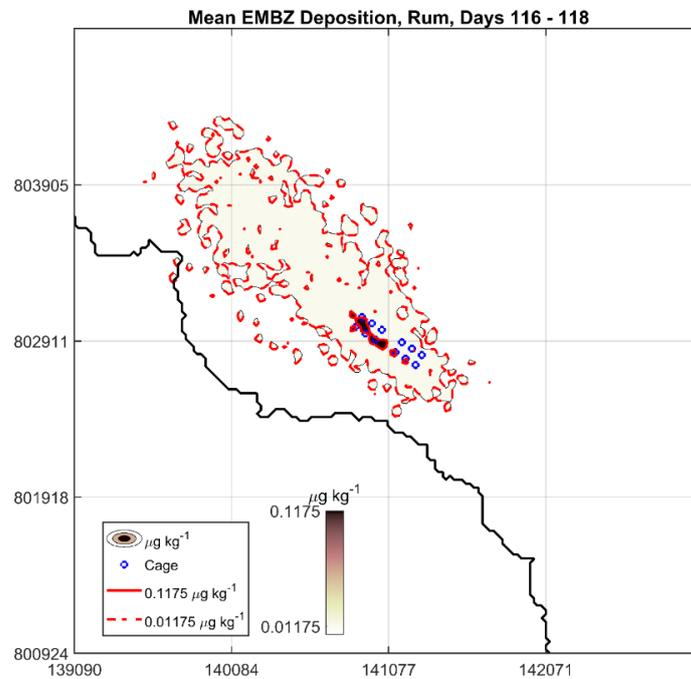
Figure 8: Predicted mean Emamectin Benzoate deposition over days 116 – 118 for the existing 12 x 120m pens at Rum following a consented treatment of 12g.
