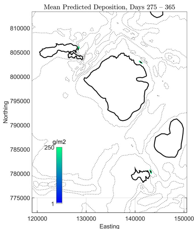
Figure 10. Predicted mean solids deposition over 90 days from the sites at Rum, Muck and the proposed site at Canna using the nominal feed rate (7 kg/tonne/day) at each site.
