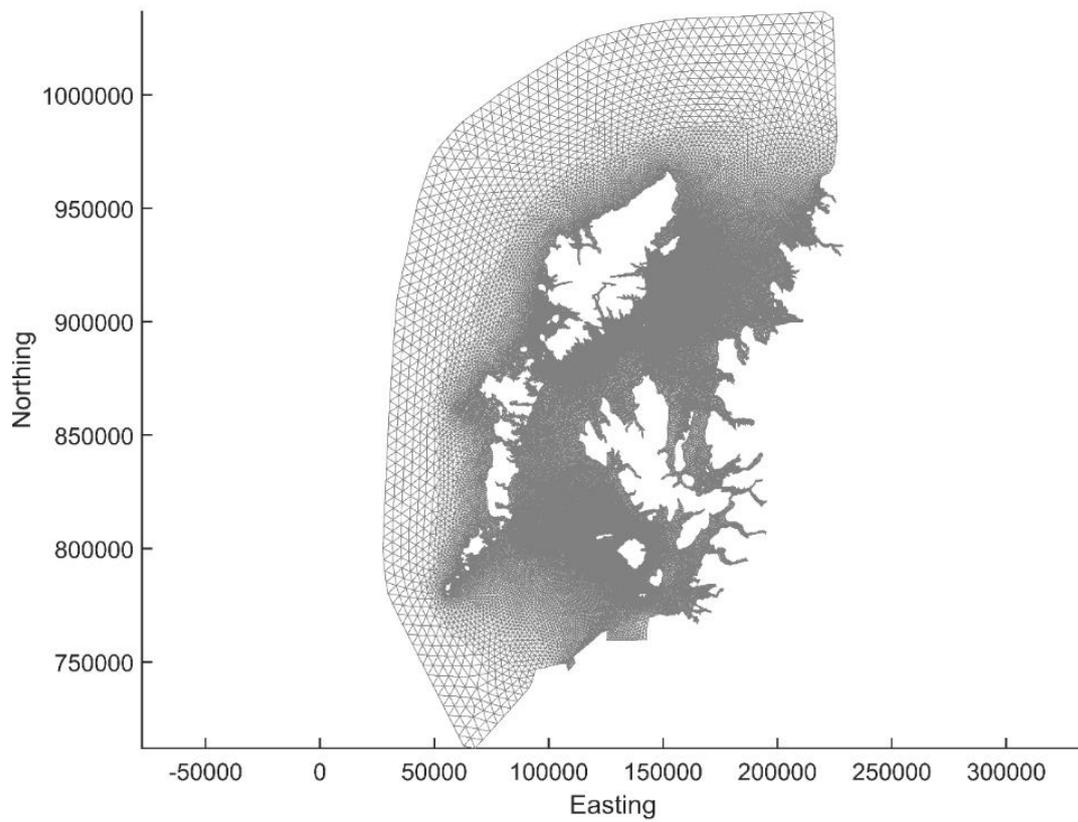
Figure 3. The modified ECLH domain and mesh used in the Rum modelling
