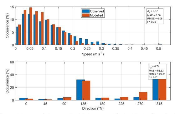
Figure 12. Histograms of observed and modelled current speed (top) and direction (bottom) at the ADCP location from August – December 2018 (ID242). Observed data are in blue, model results in red.
