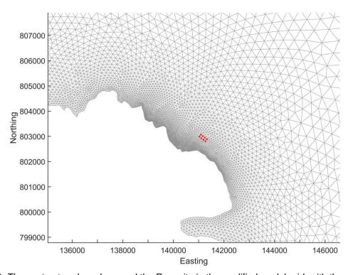
Figure 2. The unstructured mesh around the Rum site in the modified model grid, with the proposed cage locations indicated (•).
