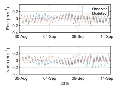
Figure 10. Comparison between observed and modelled East (top) and North (bottom) components of velocity at the ADCP location for 15 days in August – December 2018 (ID242). Observed data are in blue, model results in red.
