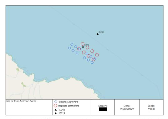
Figure 4. Locations of the ADCP deployments relative to the proposed 8 pens at the Isle of Rum site.
