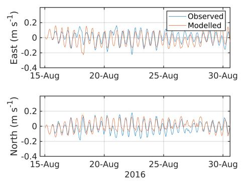
Figure 6. Comparison between observed and modelled East (top) and North (bottom) components of velocity at the ADCP location for 15 days in August - October 2016 (ID113). Observed data are in blue, model results in red.
