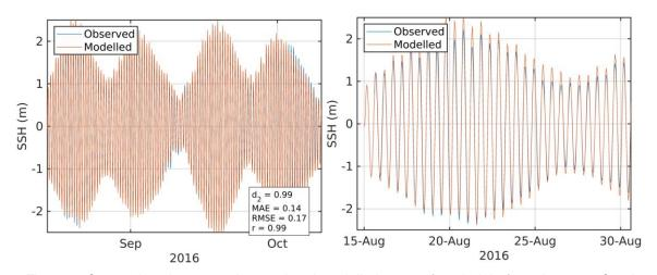
Figure 5. Comparison between observed and modelled sea surface height from August – October 2016 (ADCP deployment ID113) using model parameter values from Table 1. Both the full record (left) and a subset of 15 days (right) are shown. Observed data are in blue, model results in red.
