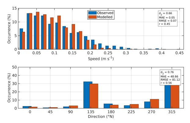
Figure 8. Histograms of observed and modelled speed (top) and direction (bottom) at the ADCP location from August – October 2016 (ID113). Observed data are in blue, model results in red.
