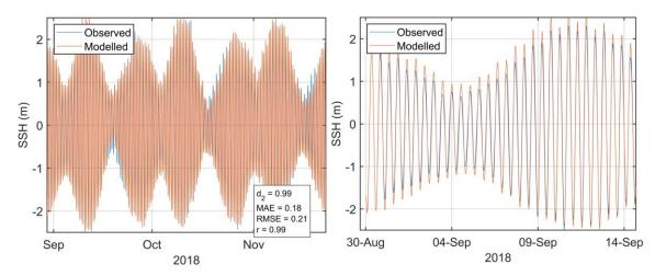
Figure 9. Comparison between observed and modelled sea surface height from August – December 2018 (ADCP deployment ID242) using model parameter values from Table 1. Both the full record (left) and a subset of 15 days (right) are shown. Observed data are in blue, model results in red.
