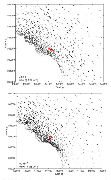
Figure 13. Modelled flood (top) and ebb (bottom) surface current vectors during spring tides. For clarity, only every 5<sup>th</sup> element of the model vectors are shown.
