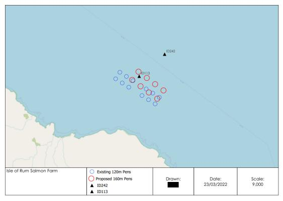
Figure 2. Existing (blue) and proposed (red) layouts at the Isle of Rum salmon farm. ADCP deployment locations are also marked with a black triangle
