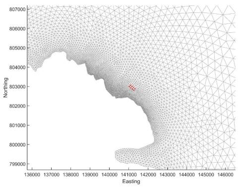
Figure 4. The unstructured mesh around the Rum site. The pen locations are indicated (o).
