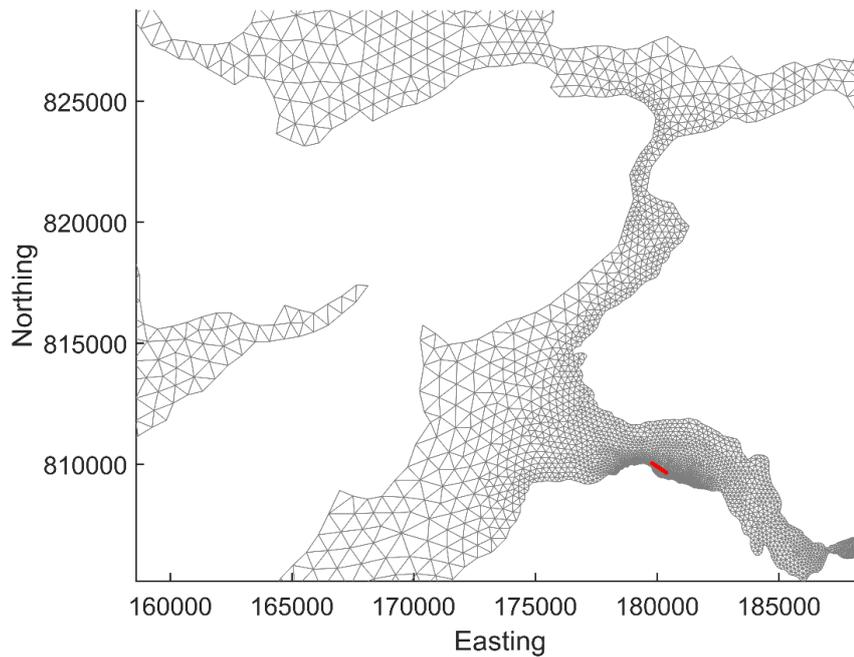
Figure 3. The model mesh in the area around the Loch Hour site. The pen locations are indicated (○).
