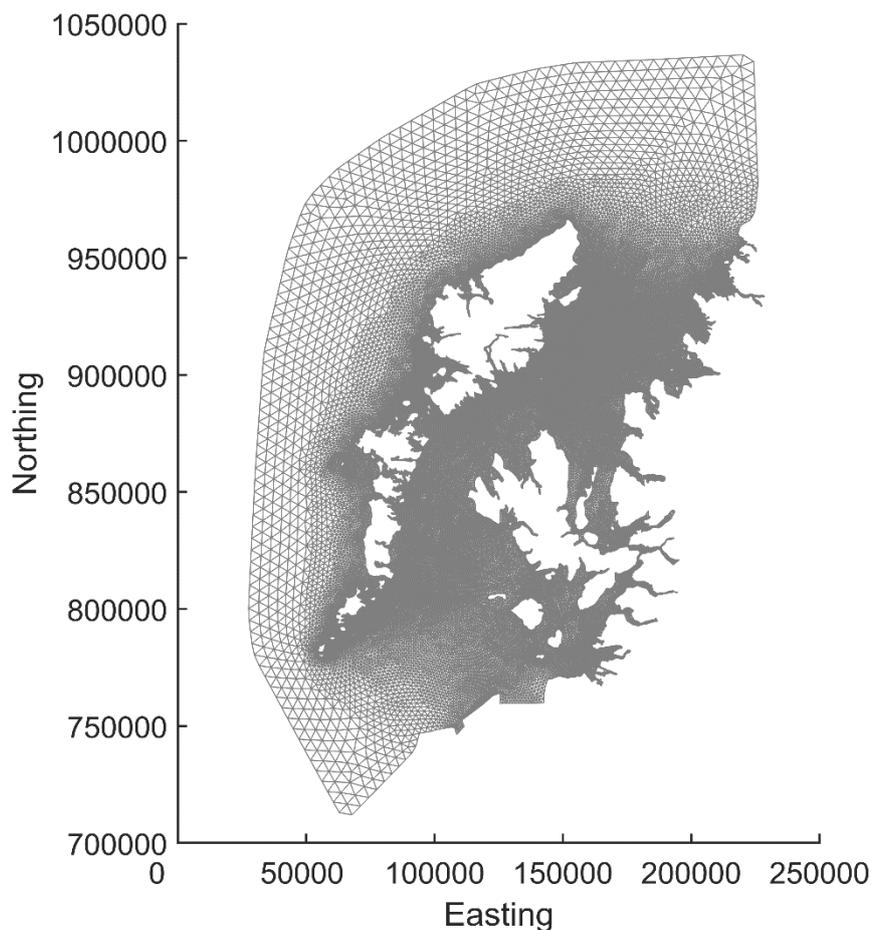
Figure 2. The modified ECLH domain and mesh used in the Loch Hourn modelling.
