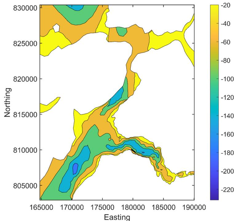
Figure 5. Localised bathymetry (m) around Loch Hour in the ECLH domain. The pen locations are marked (•).
